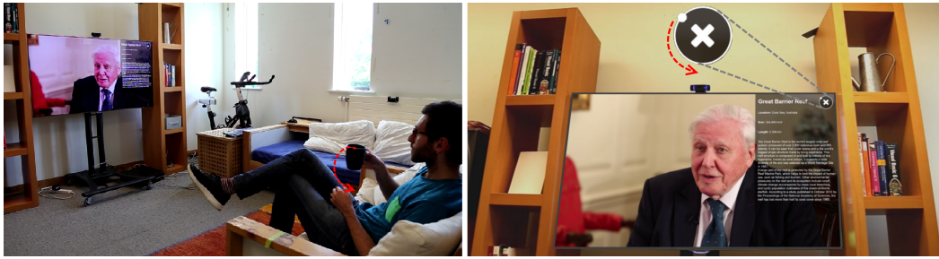
Fig. 12. TraceMatch is designed for casual motion input. A camera tracks any motion in the front off the screen and correlates it with on-screen moving control. This enables users to provide input with any part of their body, and regardless of their posture. In this scene, the user is able to close a pop-up screen on the TV by mimicking the widget’s motion with his hand even though he is holding a drink.
