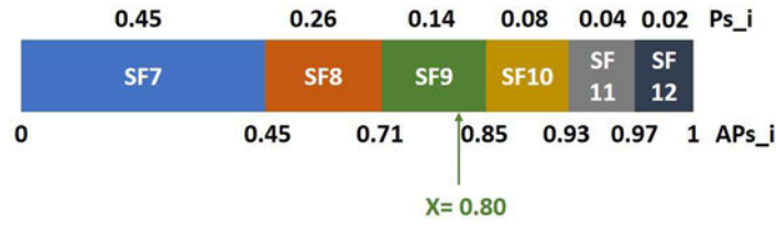
Figure 24: Example of the implemented Bit Rate Ratio Algorithm.
