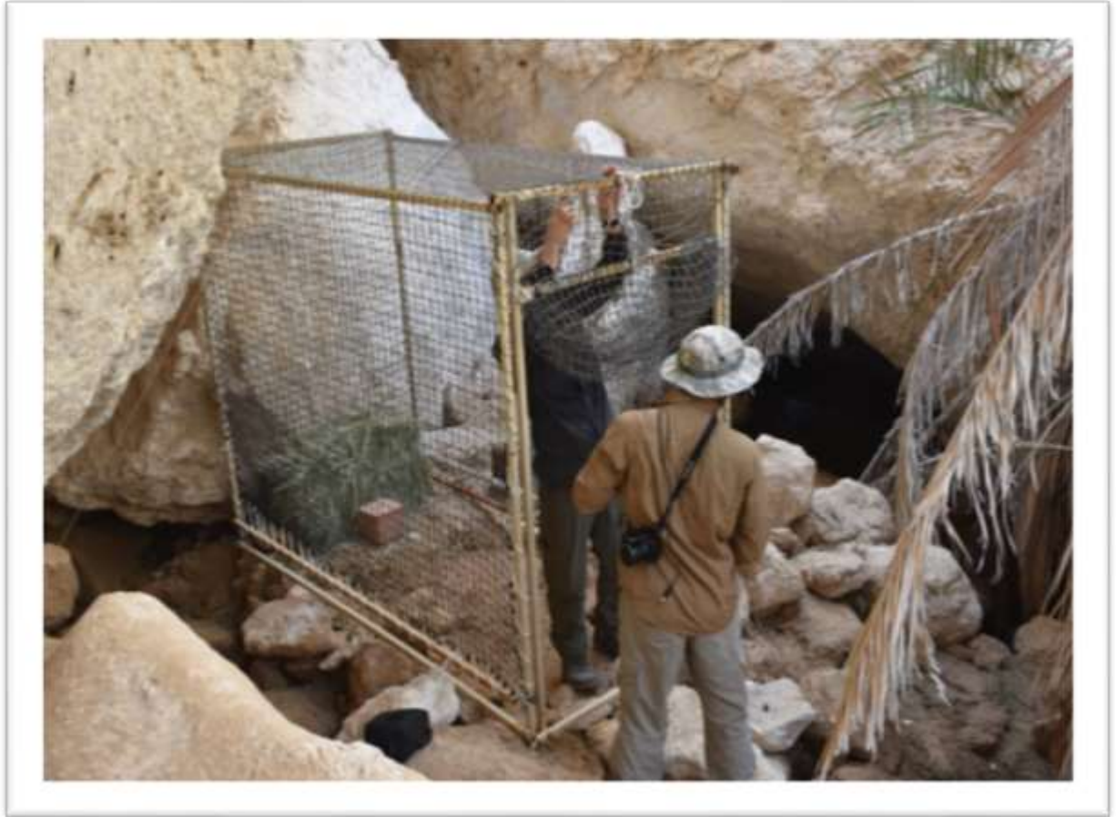
Figure 6.3. Trap used to capture wild Nubian ibex at WWR. Some hay is placed inside the trap and when animal hits the trigger the door closes. A transmission device sends a signal to alert the trapper(s) when the door is closed.
