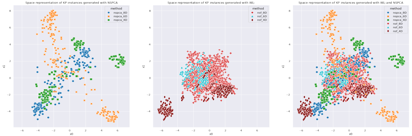
Figure 2: Instances generated for different NS algorithms represented in the same space. Yellow crosses represent the instances from NS_{PCA} projecting 8D to 2D; green squares for NS_{PCA} projecting 6D to 2D; blue circles for NS_{PCA} projecting 4D to 2D; red pluses for NS_f searching on 8D feature space; light-blue triangles for NS_f searching on 6D; and dark-red diamonds for NS_f searching on 4D.
