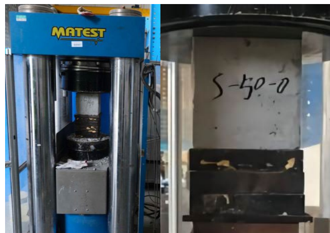
Fig. 4. Photo of the cubic compression test
