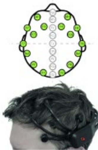
Figure 3-4- Epoc Emotic wireless, wearable EEG headset (Aspinall et al., 2015).
