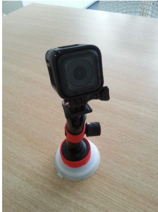
Figure 4-5 - GoPro Hero 4 Session camera mounted on a handler so it can be positioned upright on the table or held like a microphone during the walking interview.
