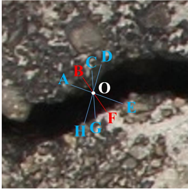
Fig. 6 Different measurement methods on the same crack
