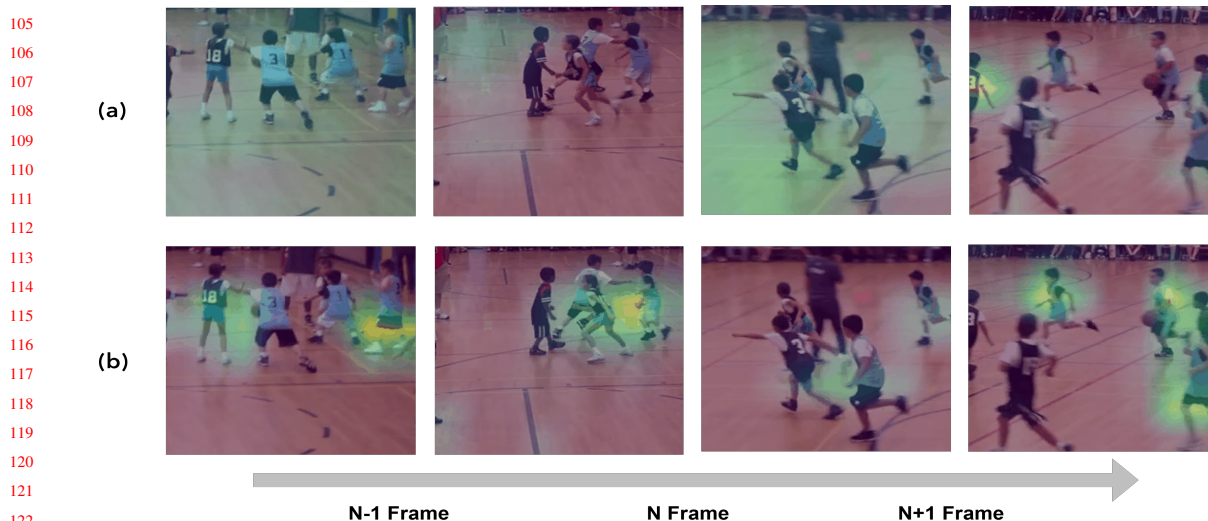
Fig. 1. An illustration of activated regions of class "playing basketball" in Kinetics400. The upper row (a): the heatmap of our baseline slowfast with T-conv fusion. (b): the heatmap of our method without fusion operations in the middle layers. For fair comparison, the backbone for both methods is slowfast R50 4×16. The time dimension increases from left to right.
