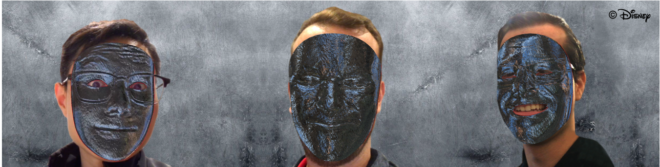
Figure 1: Guests using our Face Magic framework with themed detailed steel stylized face filters. Our system performs camera ingest to coarse mesh depth generation in .43ms, face depth smoothing in .52ms, patch based pseudo-inverse local reconstruction in 12.22ms, and our detail filter effects shaders in 1ms, leading to a total real-time processing in 15ms per frame.
