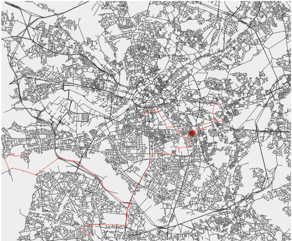
Figure 7.11: Example of the Fire department intervention problem embedded on Manchester's road network. The problem contains 1 fire and the optimised solution uses forces from 5 different sources
