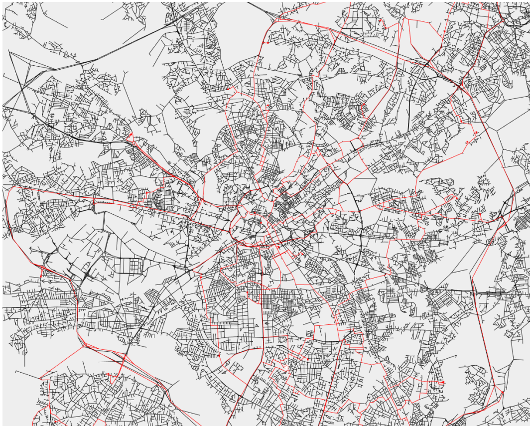
Figure 7.12: Example of the ambulance placement problem embedded on Manchester's road network. Pink lines are paths from the chosen location to the emergency location (red points) and blue lines are paths from the emergency location to the hospital.
