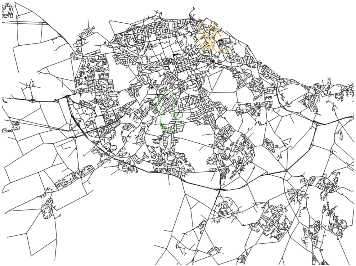
Figure 7.10: Two simple examples of the School bus problem embedded on Edinburgh's road network. In green an optimised tour and in orange a non-optimised tour. Both instances have 10 stops
