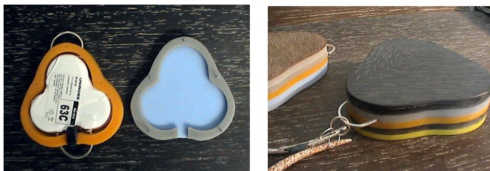
figure 5/13 battery cases with the VARTA coin cell arrangement in place
