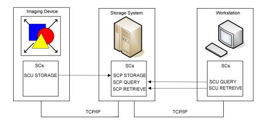
Figure 2.1: DICOM Distributed Model and Service Classes
