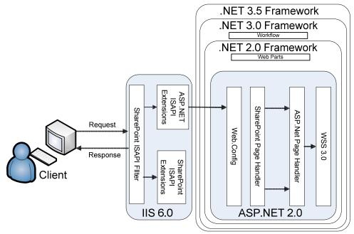
Figure 3.1. Typical request response ASP.NET and WSS
