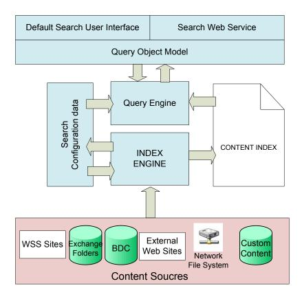
Figure 3.4 Simplified view of MOSS search and indexing architecture
