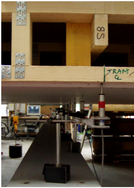
Figure 4.18: LVDTs at mid-span
