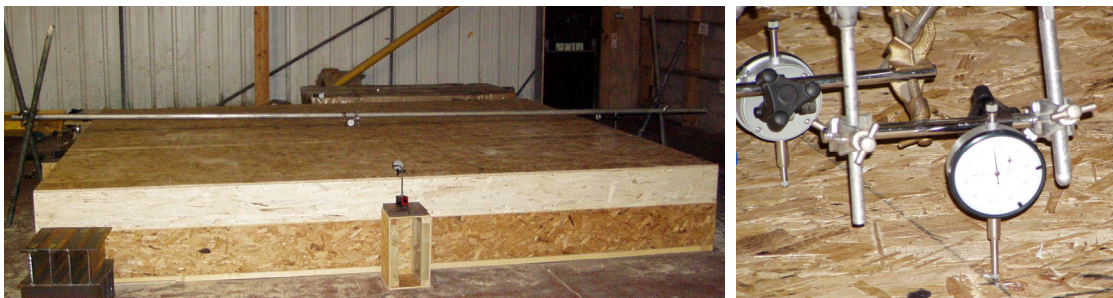
(a) Dial gauges in the centre and at the edges
