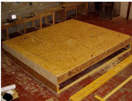
(e) Complete floor with OSB deck
