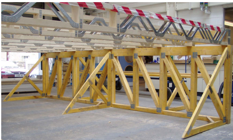
(a) Metal-web joists on supporting truss
