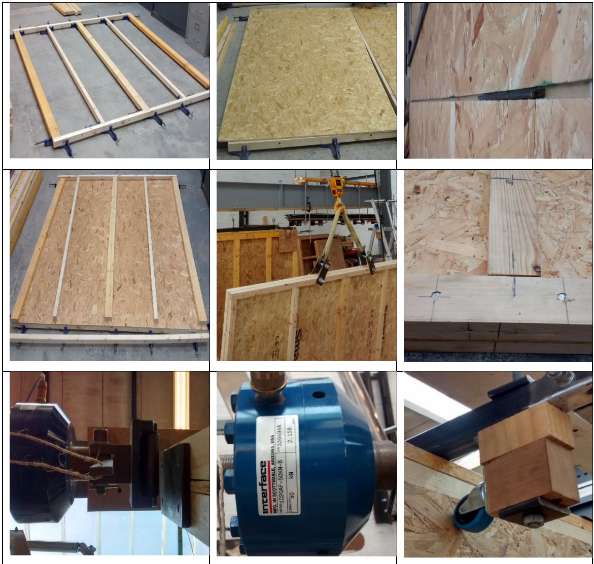
Appendix 6.4 Typical example of wall Type 1 with 150 mm nail spacing
