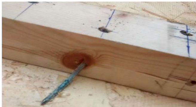
(b) Bend out of ring shank nail using nail gun
