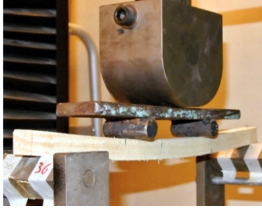
Figure 9: Four-point bending tests to assess the characteristic bending strength [11].
