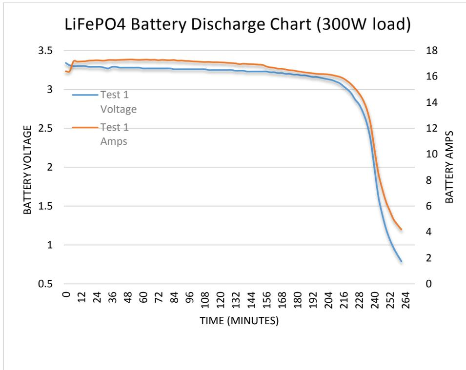
**Figure 61 LiFePO<sub>4</sub> discharge curve (experimental)**
