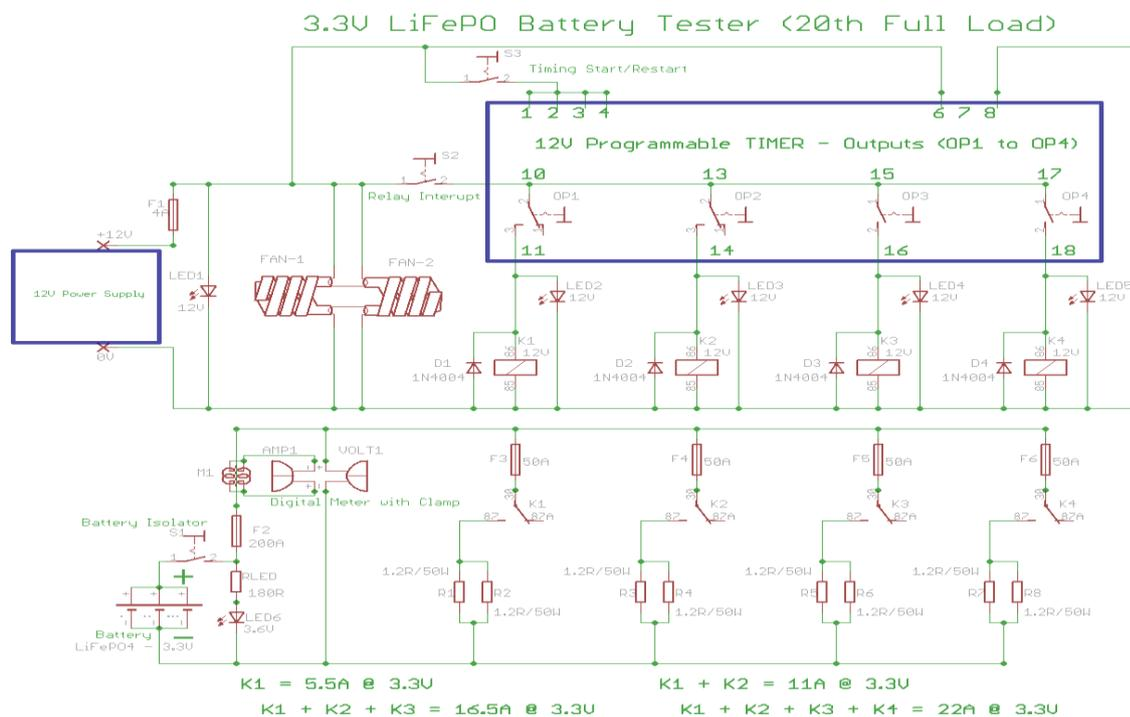
**Figure 62 Variable Load Battery Tester schematic**
