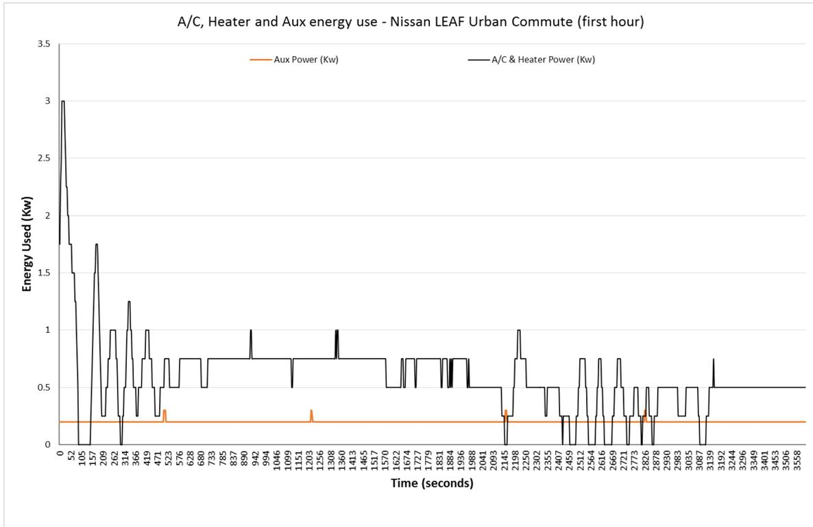
**Figure 104 A/C and auxiliary energy use**
