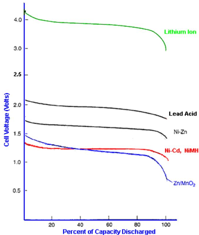
**Figure 59** Differing cell chemistry discharge behaviour
