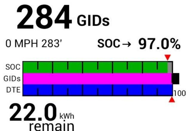
**Figure 85      High Voltage Traction Battery information from CANBUS port**
