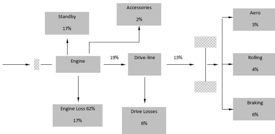
**Figure 11 Energy losses in an automobile**
