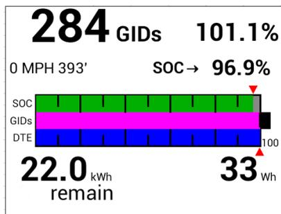
**GIDS** = Value representing state of charge of the battery. 1 GID is equivalent to 75-78Wh of available energy therefore this statement is correct and in keeping with the traction battery energy capabilities.
