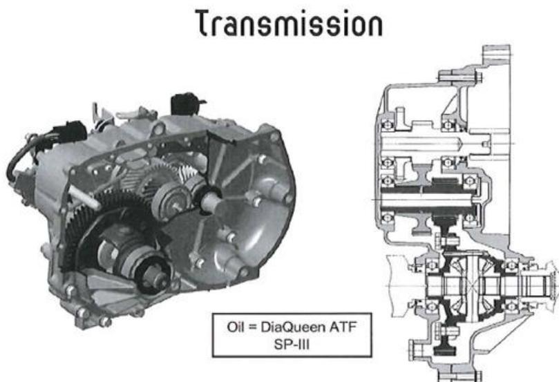
**Figure 28 Transmission general layout**
