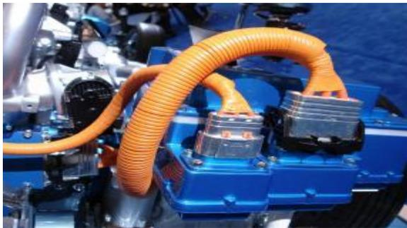
**Figure 30** Cable colour coding
