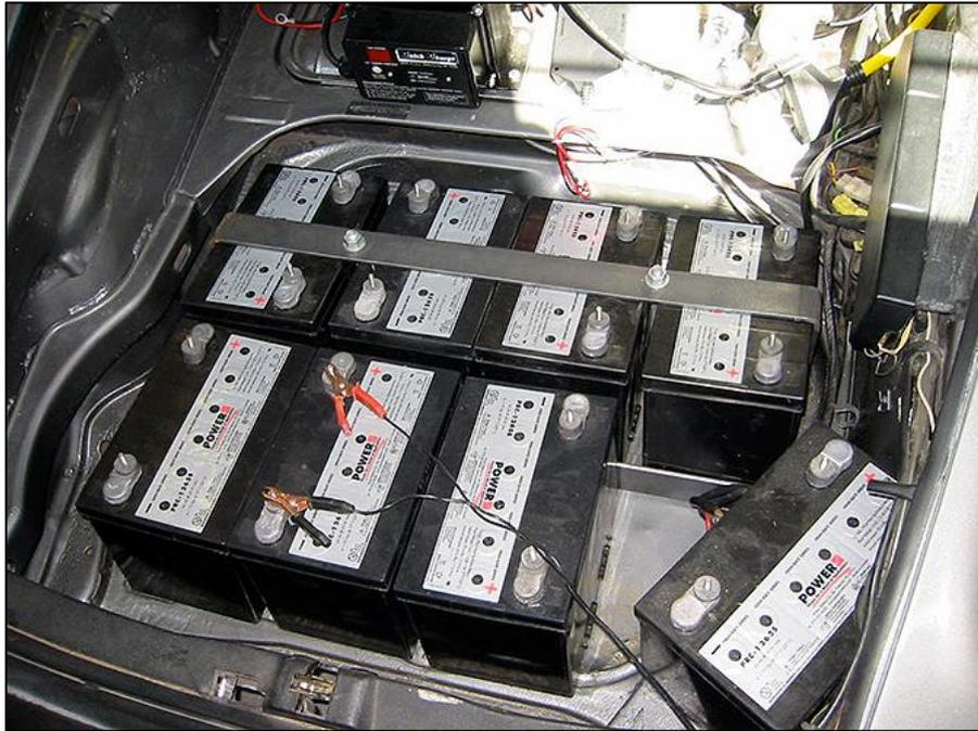
**Figure 39** Edinburgh College own vehicle - multiple lead acid battery pack
