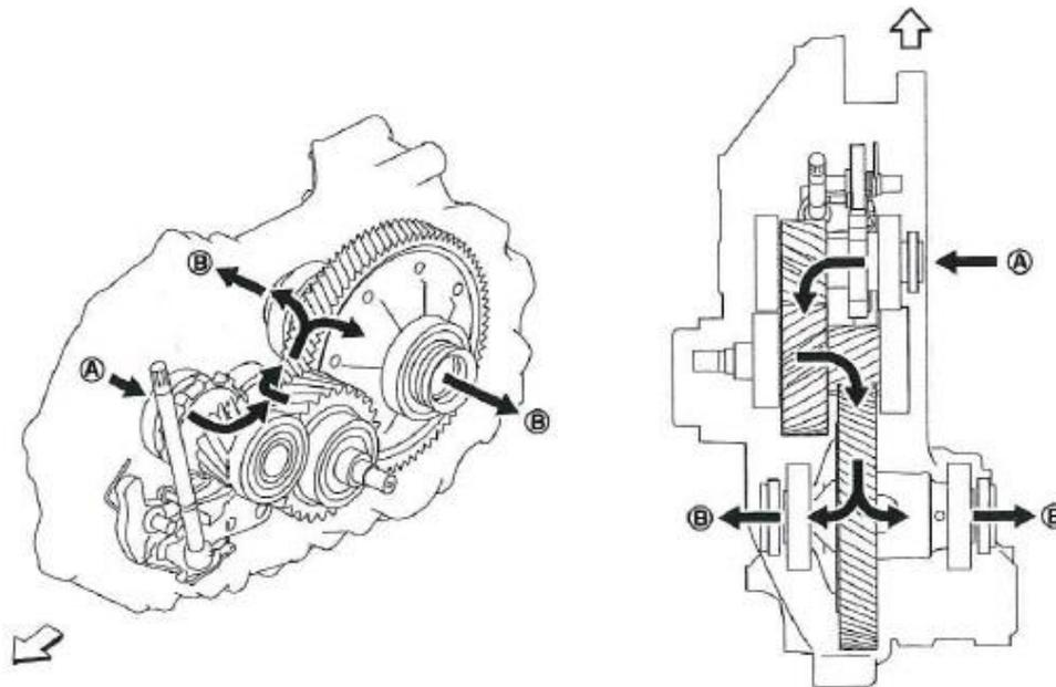
**Figure 35** Transmission power flow
