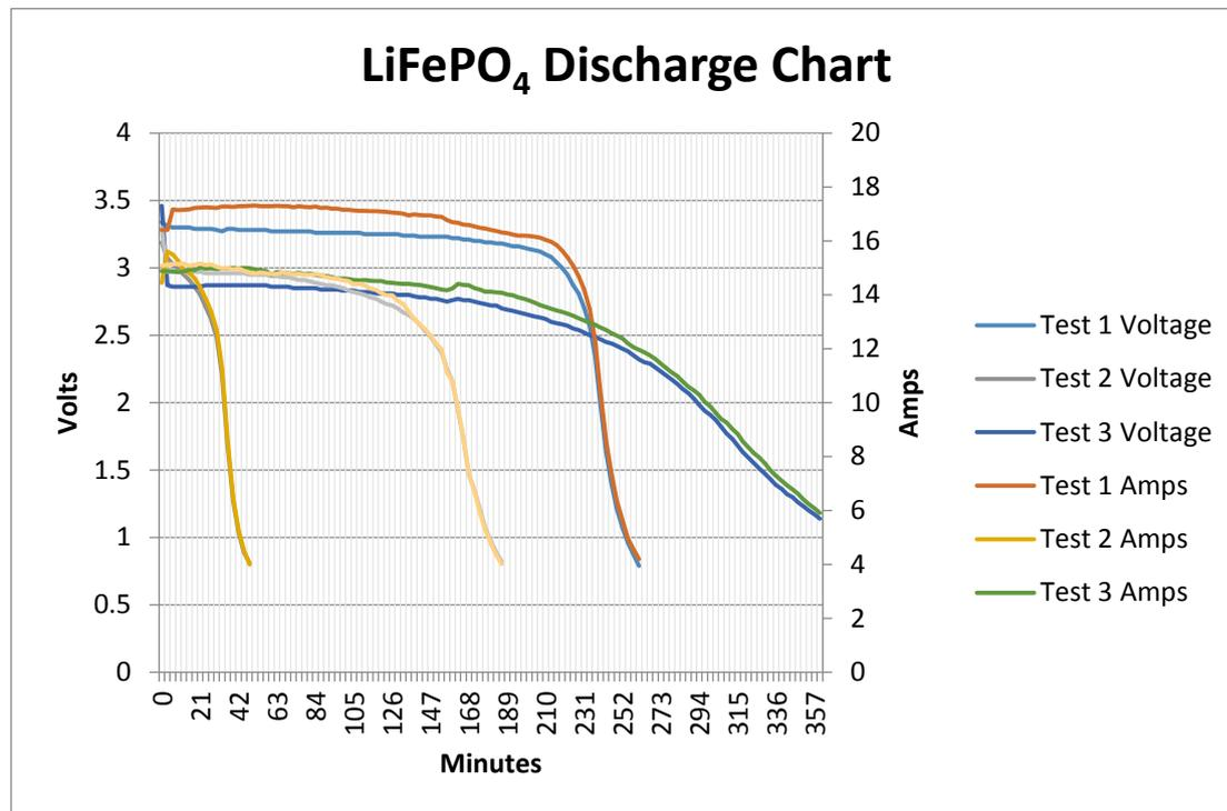
**Figure 63** LiFePO<sub>4</sub> discharge curve (test – manufacturer CALB)
