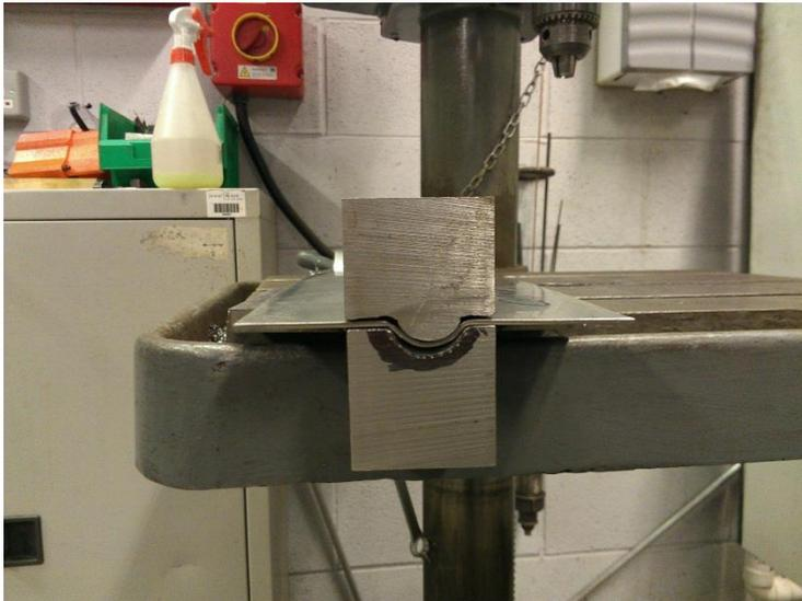
**Figure 128** Forming door for cable exit
