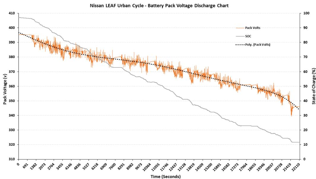
**Figure 109 Battery pack voltage discharge curve for the urban drive cycle**
