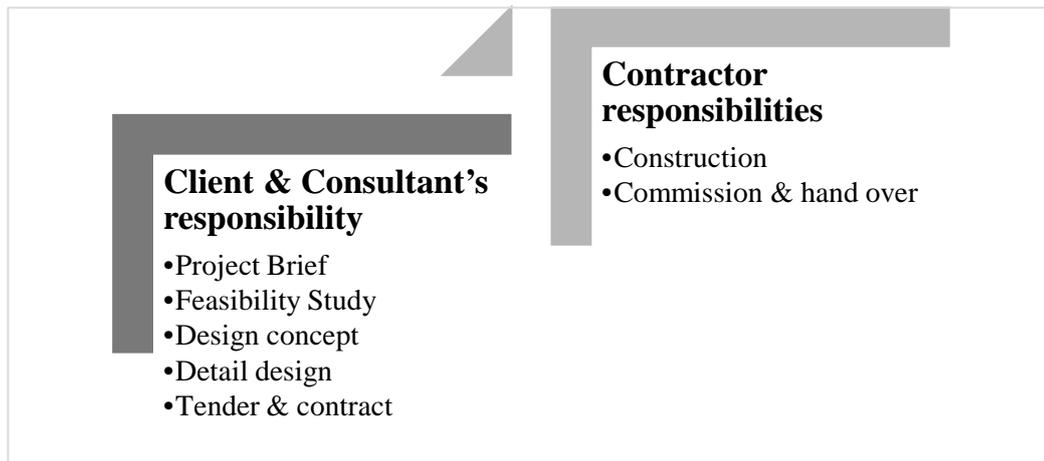
**Figure 3-2 Showing the process of the traditional Procurement System**
