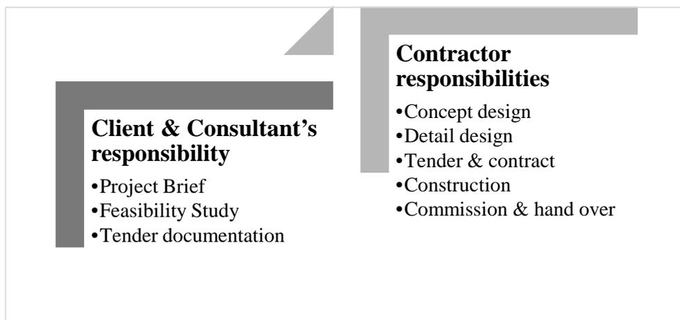
**Figure 3-3 Showing the Process of the D&B Procurement System**
