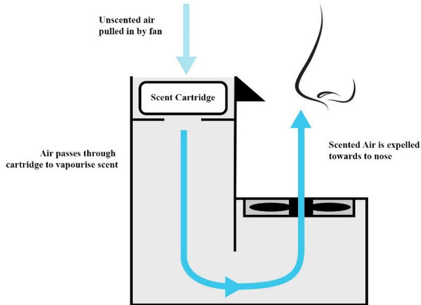
*Figure 19: Cross section of prototype demonstrating the vaporisation of the scent and how it is delivered to the nose using the fan.*
