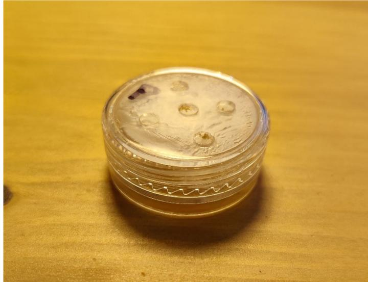
*Figure 16: The developed olfactory 'cartridge' Note there are matching holes drilled in the bottom to facilitate the passage of air.*
