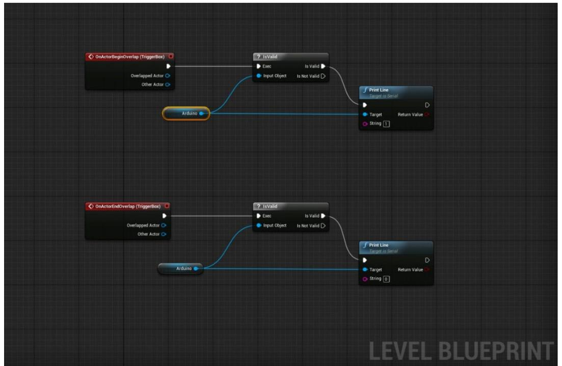
**Figure 23:** A sample script for triggering a single scent release. The script sends a value of 1 when inside the trigger area and a value of 0 when outside.
