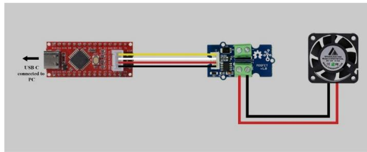
*Figure 17: Circuit Diagram of Prototype.*
