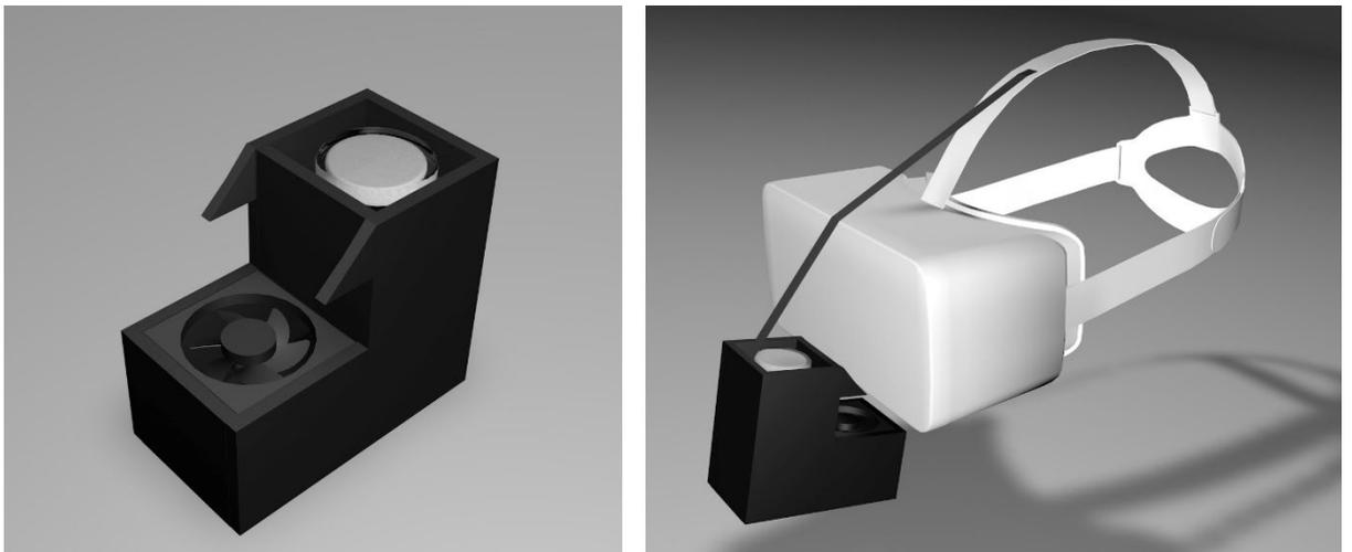
*Figure 20: 3D Renders of the prototype device and a demonstration of how it attaches to the HMD (HMD Model created by VitaminCo (2018)).*
