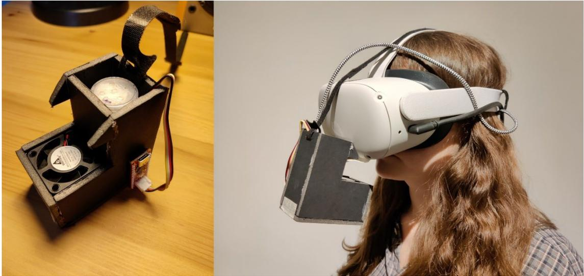
*Figure 21: Left: The physical prototype device demonstrating how the Seeduino nano is attached. Right: The prorotpye attached to an Oculus Quest 2*
