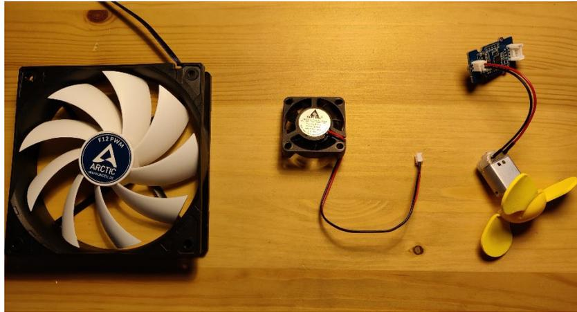
*Figure 15: Left to Right: 120mm 12V Fan, 40mm 5V fan, GROVE 5V Mini fan.*
