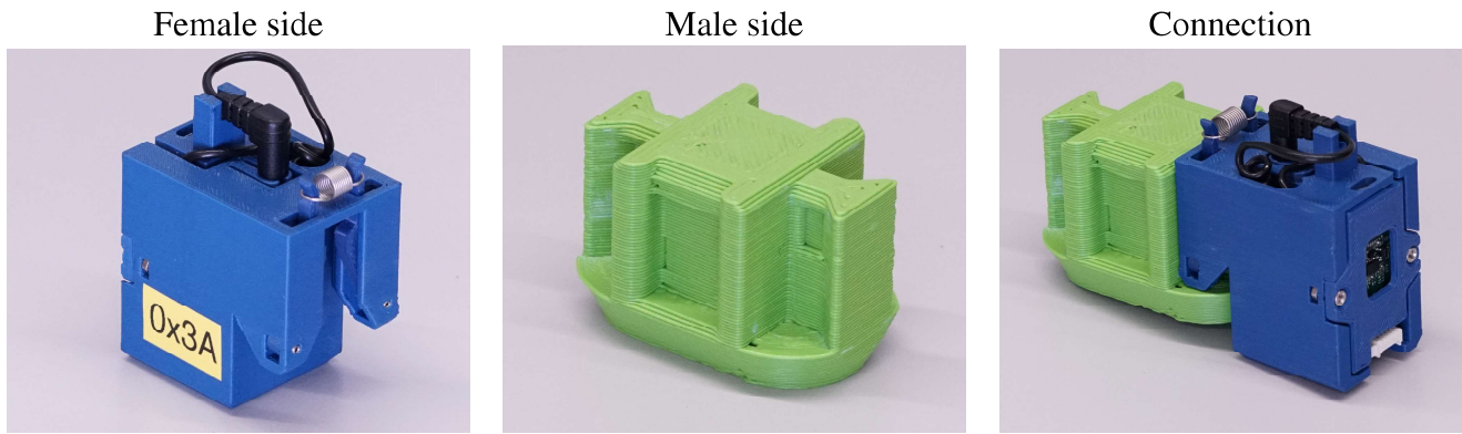
Figure 5. This figure shows the mechanical connector used in the ARE platform. The female side (left) uses two sprung arms to engage with the indentations on the male side (middle) to form the final connection (right).
