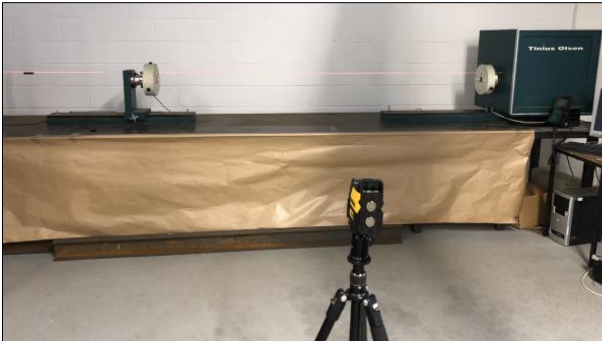
Figure 6-6: Alignment marking torsion machine chucks using laser level and wall reference marks prior to beam installation.
