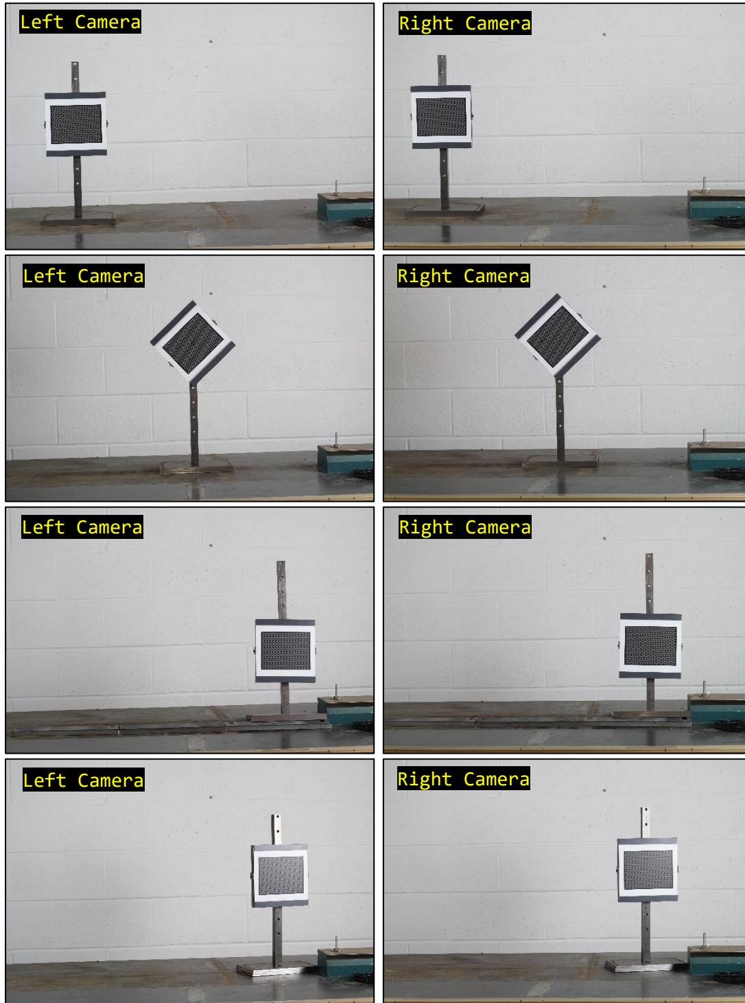
Figure 4-10: Calibration images taken in various poses – left camera images taken from 50 cm horizontally apart from right camera images.
