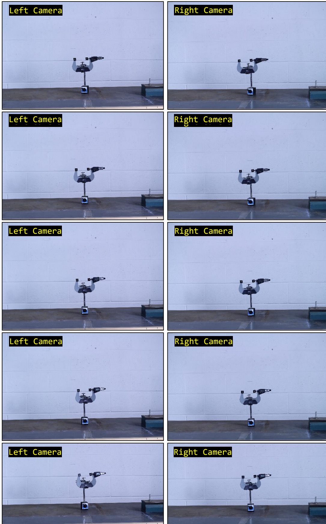
Figure 4-14: Micrometre pose cycles, left-facing to right-facing - left camera images taken from 50 cm horizontally apart from right camera images.
