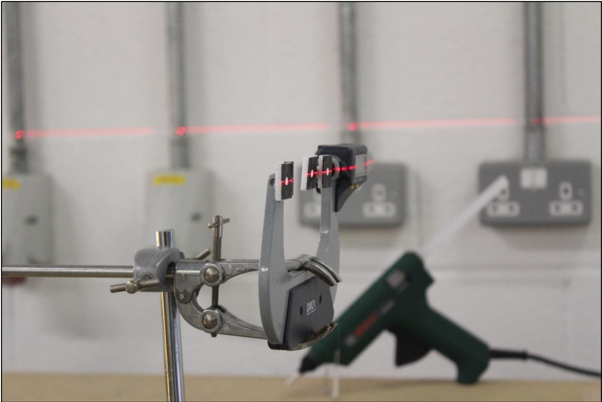
Figure 6-11: Micrometre target alignment using laser level.
