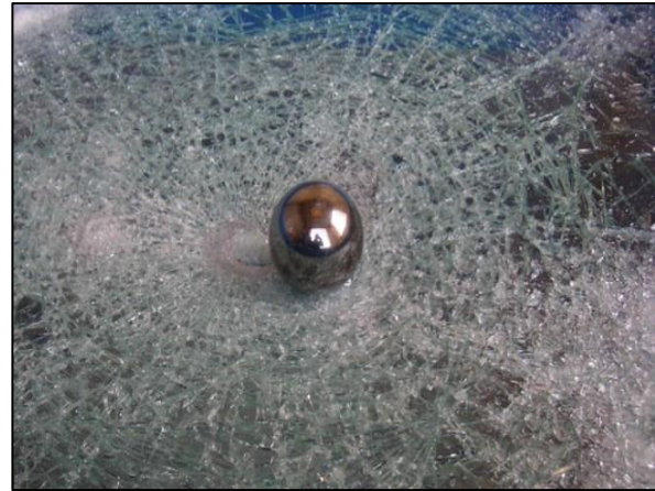
Figure 2-12: Fractured but not perforated laminated glass after hard body drop test [8].
