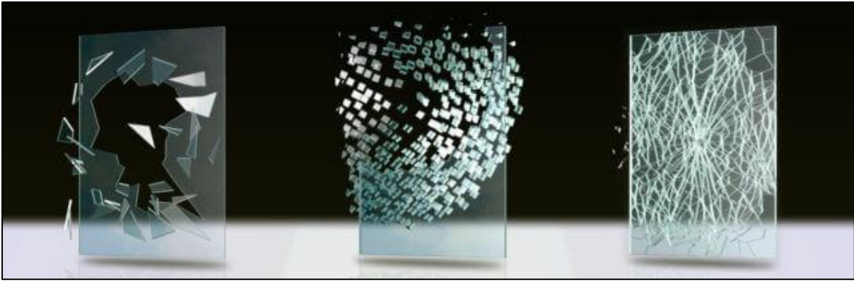
Figure 2-9: Fracture of main glass types: annealed (left), tempered (centre), laminate (right) ( www.brennancorp.com ).
