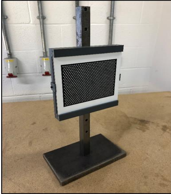
Figure 4-7c: Installed calibration unit.
