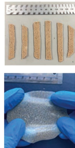
Fig. 6. Engineering tensile stress versus engineering tensile strain curve for the composite film; the two embedded images show the tensile samples and the composite film before testing.
