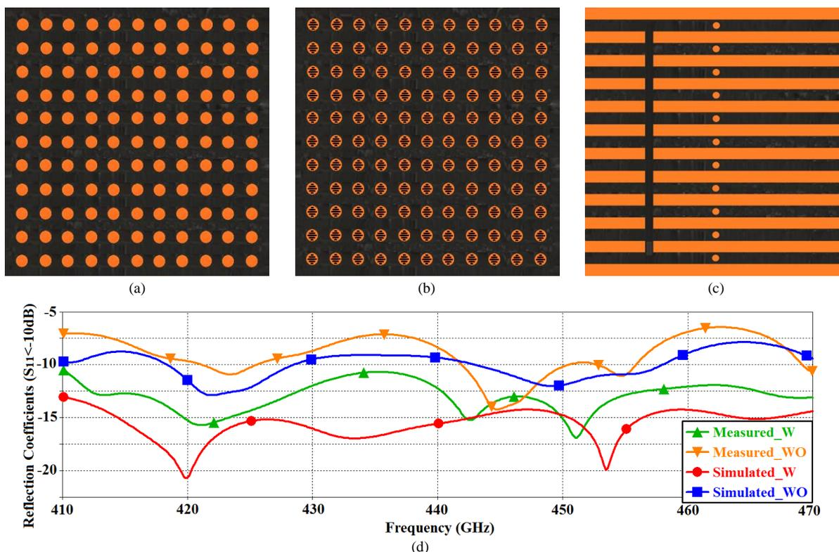
Fig.2. Fabricated prototypes of the reference, i.e. without (WO) metasurface slots, and the proposed, i.e. with (W) metasurface slots, on-chip antennas. (a) Top-view of the reference on-chip antenna, (b) top-view of the proposed on-chip antenna, (c) back-view of both on-chip antennas, and (d) the simulated and measured reflection-coefficient response.
