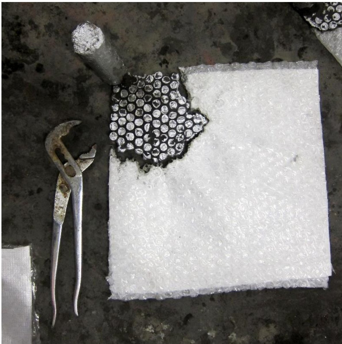
Fig 3. Incomplete cast with sprue, as an indicator of its making (Lambert, 2015).
