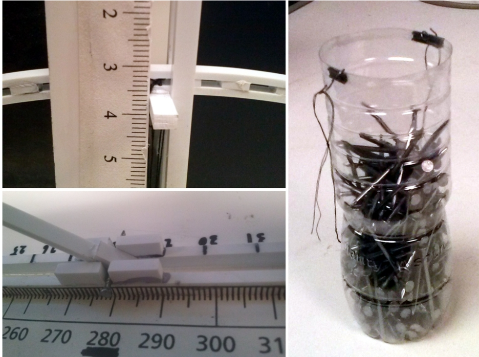
Figure 3.18: Set-up for the experimental test: the load is applied by increments of 2.18 g, by placing nails into a basket hanging underneath the structure and tied to the arch midspan by wire.
