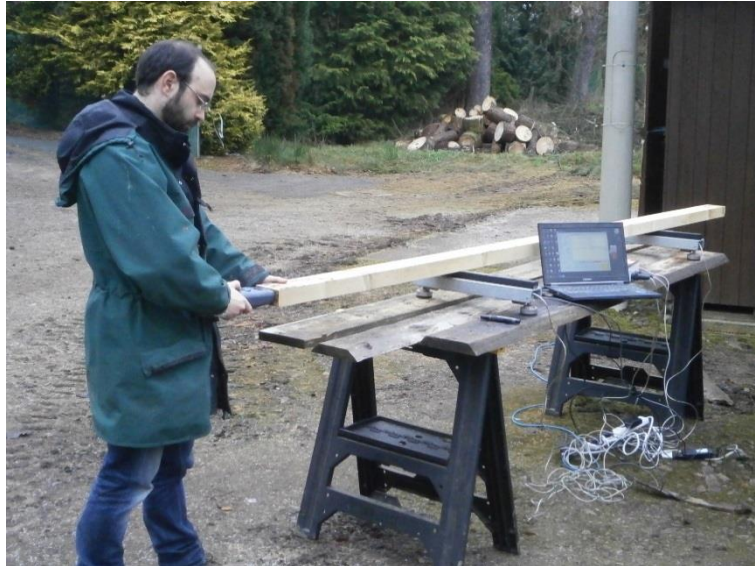
Figure 5-4. Acoustic measurement on sawn timber.
