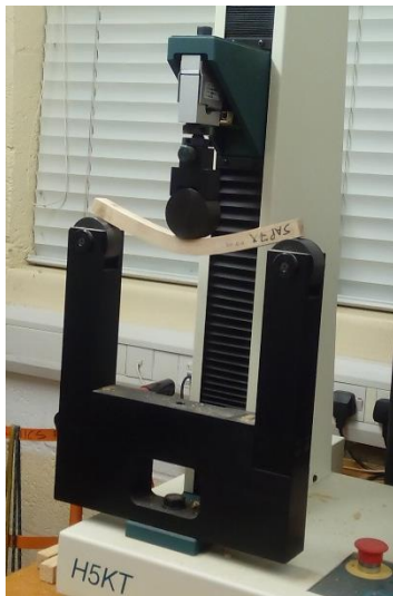
Figure 2-15. Small clear specimen under a test load.
