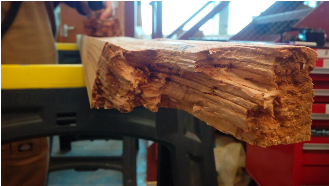
Figure 2-6. Collapse in a tested (broken) piece of western red cedar.
