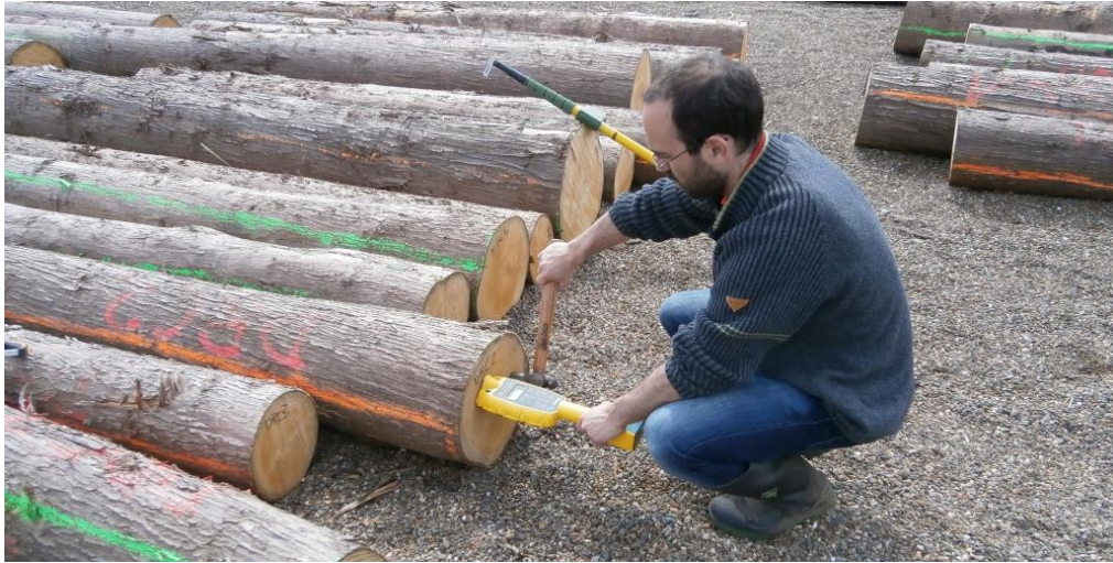
Figure 5-3. Measurement of resonance in logs.
