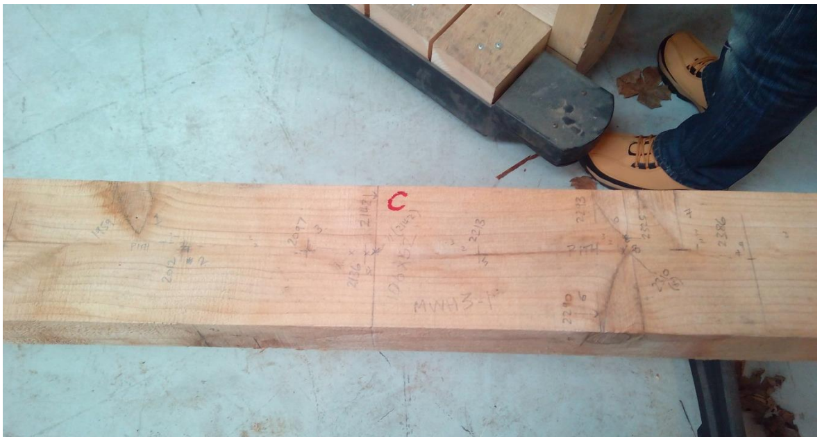
Figure 2-8. Section selected for destructive testing and knot assessment.
