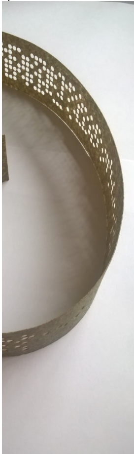
Figure 7. Laser cut ribbon made with recycled wool and PLA Source: TDRG - Source
