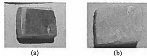
Fig. 4 Marble samples for SEM and EDX testing: (a) fully dirty sample and (b) fully clean sample.
