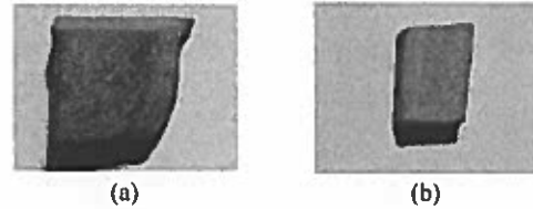
Fig. 2 Yellow sandstone samples for SEM and EDX testing: (a) fully dirty sample and (b) fully clean sample.
