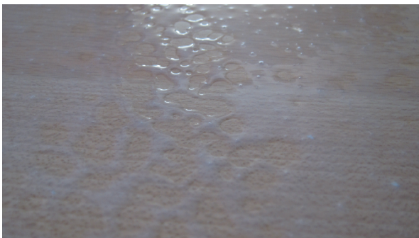
Figure 2. A laminated wood bedside table coated with NanoCote HD-WR (before curing). Close-up view showing a particularly poorly wetted area.
