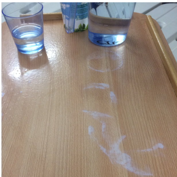
Figure 7. A laminated wood bedside table coated with NanoCote HD-WR after curing, on which some water had made contact with the surface.
