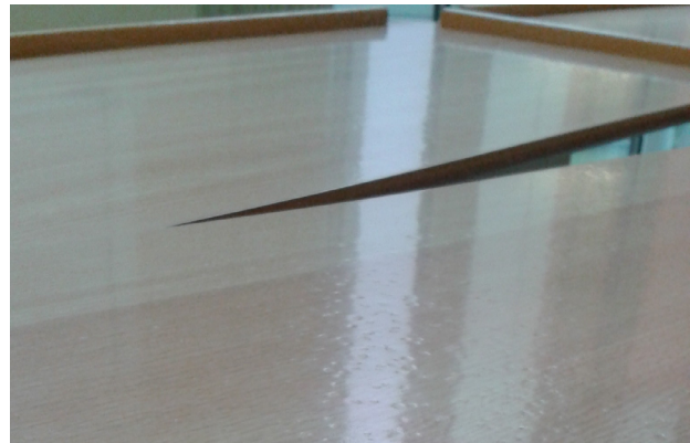
Figure 6. Laminated wood bedside tables coated with NanoCote HD-WR (after curing), showing a somewhat smoother final finish, but cratering is still obviously present.
