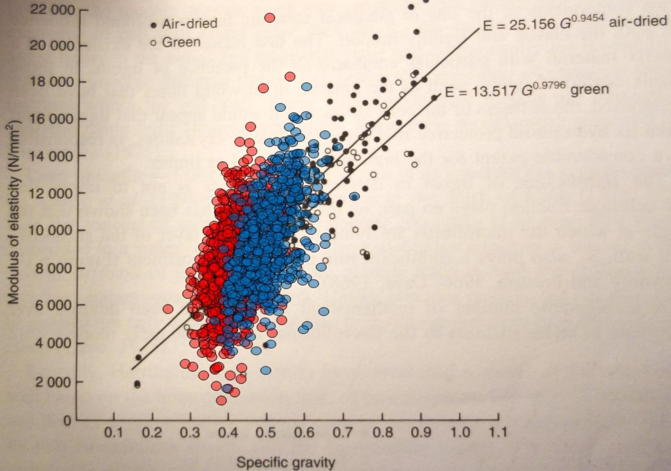
Figure 6.9 Effect of specific gravity on the longitudinal modulus of elasticity for over 200 species of timber tested in the green and dry states. (© BRE)
