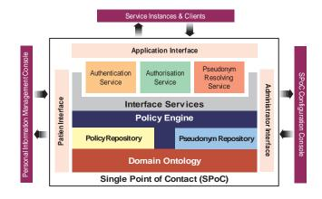
Fig. 1. The internal architecture of a SPoC
