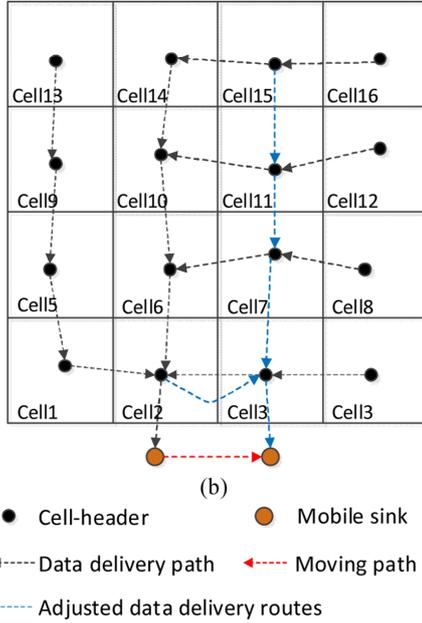
When the mobile sink moves to Cell 3, the cell-header in Cell 3 becomes a new OCH and execute Rule 2 to update the routes from downstream cell-headers to the current OCH. The downstream cell-header means cell-headers, i.e., 7, 11 and 15. Furthermore, the current cell-header executes Rule 3 to update the routes from the previous OCH to the current OCH. Blue arrows represent adjusted data delivery routes. The specific algorithm is also shown in Algorithm 1.
