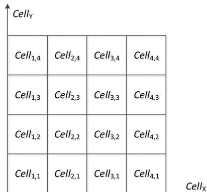
Based on the optimal number of cells which has been calculated using equation (1), we can get the side length of cells as  $L/\sqrt{K}$ , where  $L$  is the side length of the virtual grid. Then each node can get its own serial number,  $\text{Cell}_{x,y}$  using equation (2).
