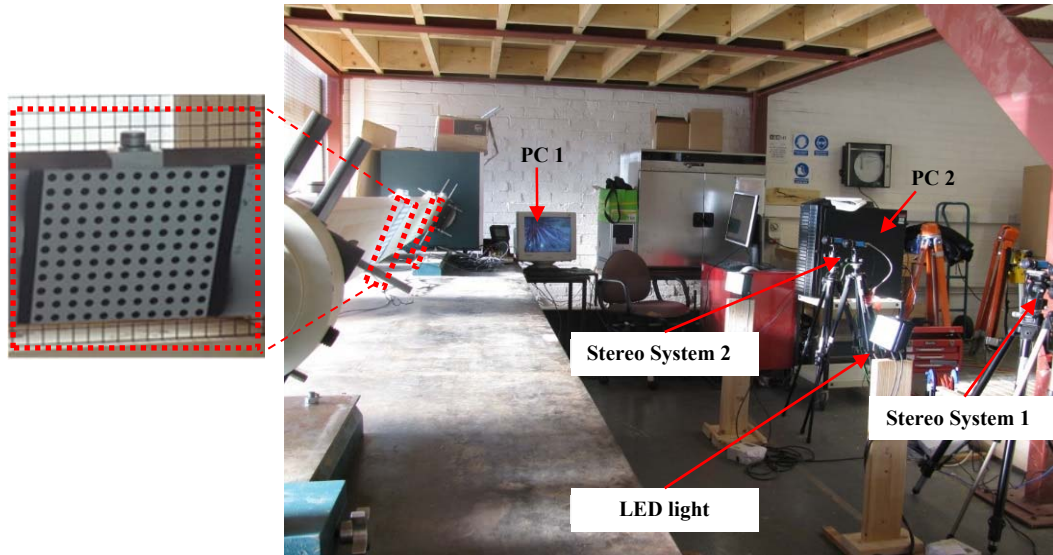
Figure 5-31: Image of experimental setup of the torsion test (left) and a detail of the photogrammetric pattern (right).
