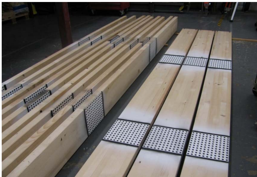
Figure 5-27: The glulam samples after being painted with the photogrammetric patterns.
