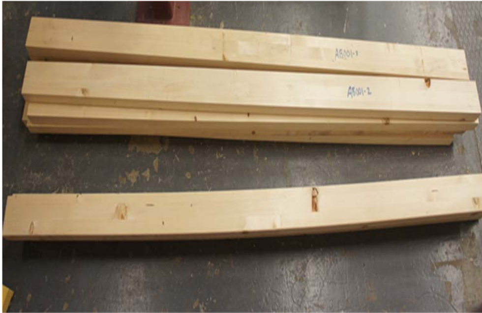
Figure 5-1: Glulam timber specimens for torsion tests.
