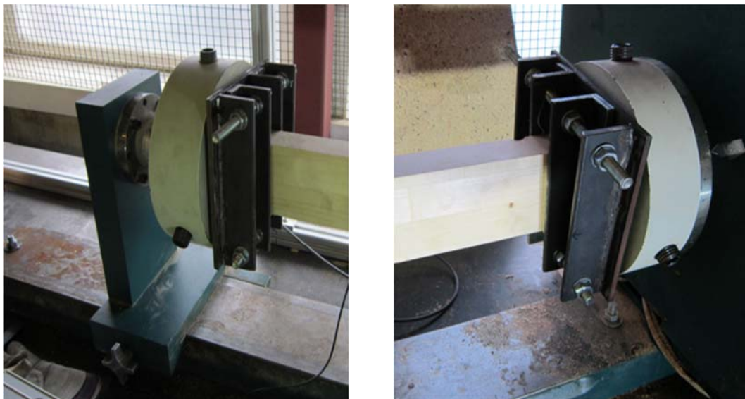
Figure 5-6: Clamps of the torsion tester at the fixed end (left) and at the rotating end (right).
