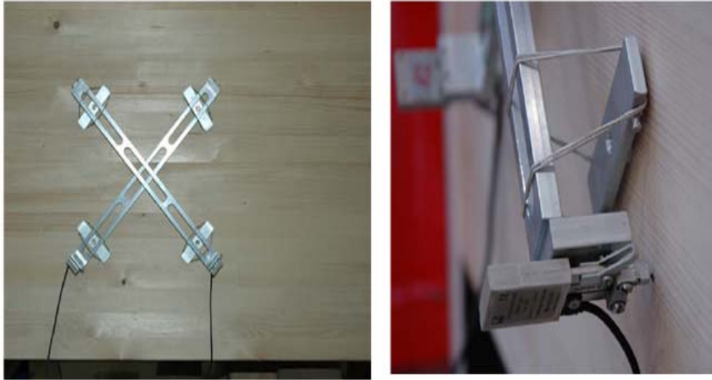
Figure 2-6: Example of the shear field test apparatus fixed on one of both sides (BS EN 408:2010).
