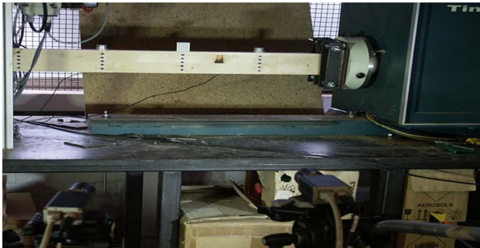
Figure 5-12: Image of the test setup of the specimen on the torsion machine with instrumentation.
