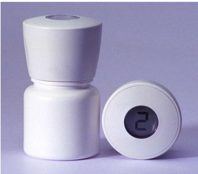
Figure 3.5. Medication Event Monitoring System (Ardex, 2005)
