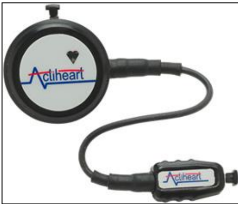
Figure 3.3. The Actiheart monitor
