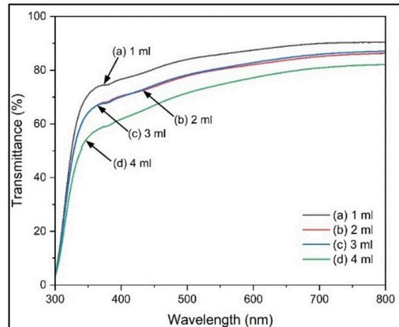
Figure 3: The graph of optical transmittance against wavelength of a-C thin films
