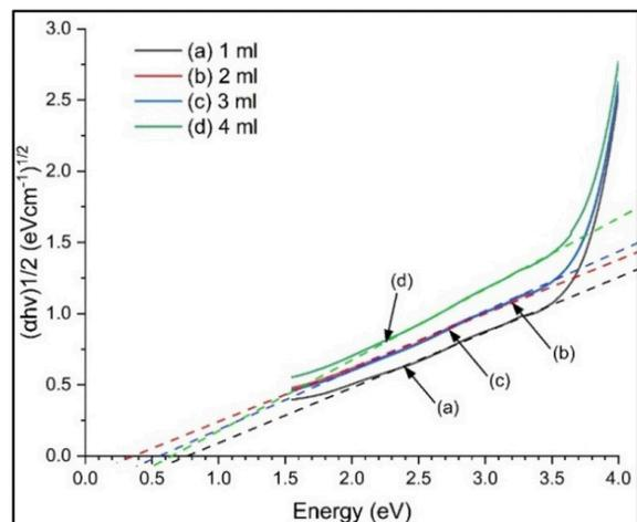
Figure 4: The graph of Tauc plot of against photon energy for a-C thin films
