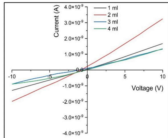
**Figure 5:** The I-V characteristic curve of a-C thin films
