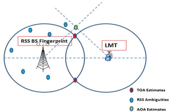
Figure 8. Combination of ToA, AoA and RSS fingerprints
