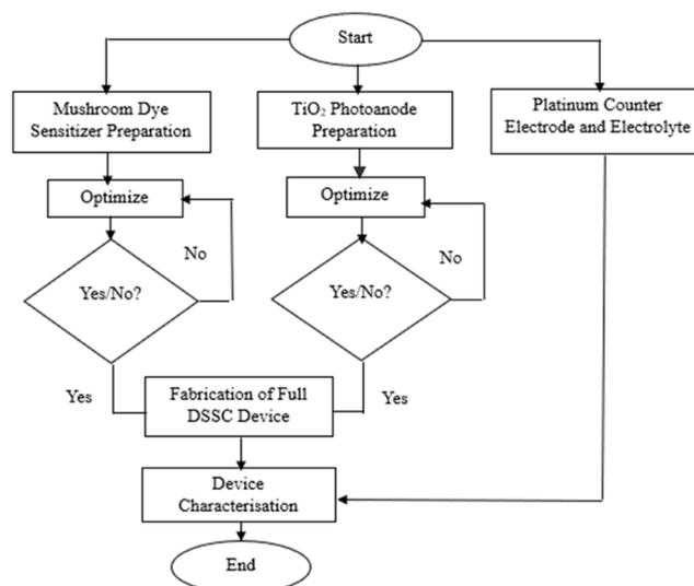
Fig. 1. Flowchart of the DSSC Fabrication.
