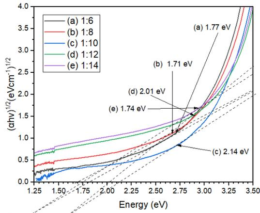
Fig. 3. UV Tauc Plot for PFOM dye.
