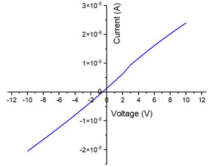
Fig. 4. I-V measurement plots of TiO<sub>2</sub> photoanode after being immersed in PFOM dye.
