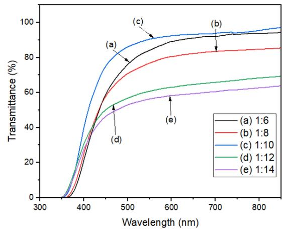
Fig. 2. UV-Vis transmittance spectra for PFOM dye.
