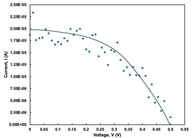
Fig. 5. J-V Characteristics for FTO/TiO<sub>2</sub>-PFOM/electrolyte/Pt.
