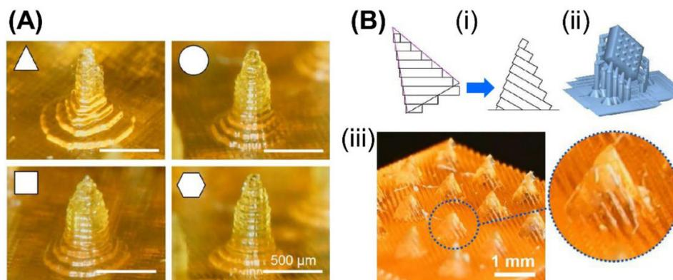
**Fig. 3.** Microneedle array (MNA) fabrication utilizing combined 3D printing and micromolding, (A) 3D modeling of master MNA using computer-aided design (CAD) software, (B) 3D printing of the designed MNA, (C) replication of the master mold, (D) arrangement of multiple master molds on a holder, (E) manufacture of MNA fabrication mold by polydimethylsiloxane (PDMS), (F) drug loading on the tip of the fabricated MNAs; reprinted with permission from Elsevier (Balmert et al. 2020).
