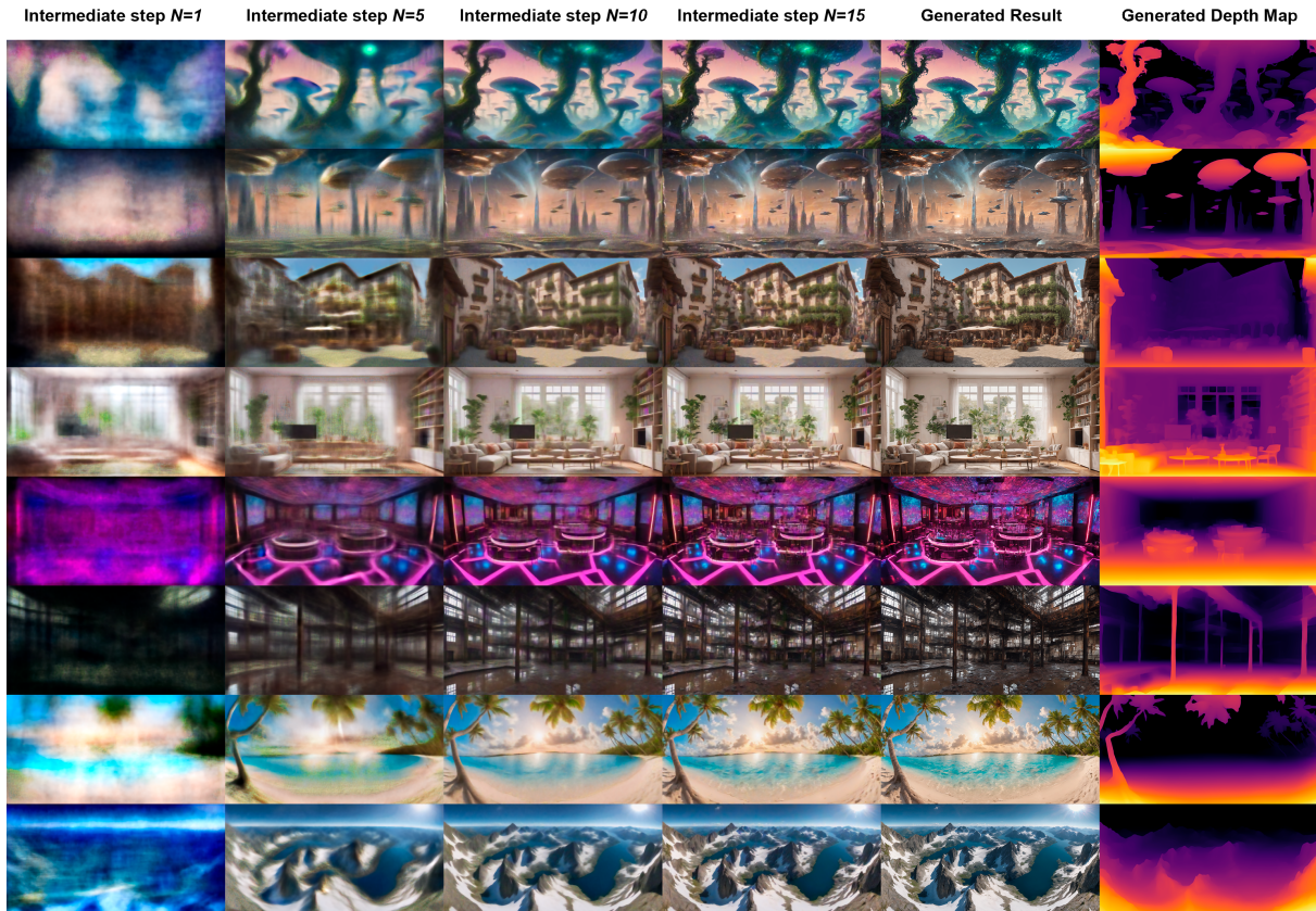
FIGURE 4. Illustration of the process for generating environments with real-time access to live previews of the images. Intermediate samples are displayed at computation steps 1, 5, 10, 15, and the final output. A corresponding depth map is generated using DepthAnything [11], providing additional spatial information of depth-based parallax 3D rendering in VR.
