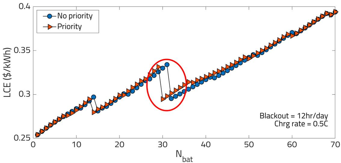
**Figure 10.** Levelized cost of energy as a function of the number of batteries in the system. The priority load management causes the battery replacements to reduce around  $N = 14$  and  $N = 30$  (indicated with the red circle). This causes drop in LCE.
