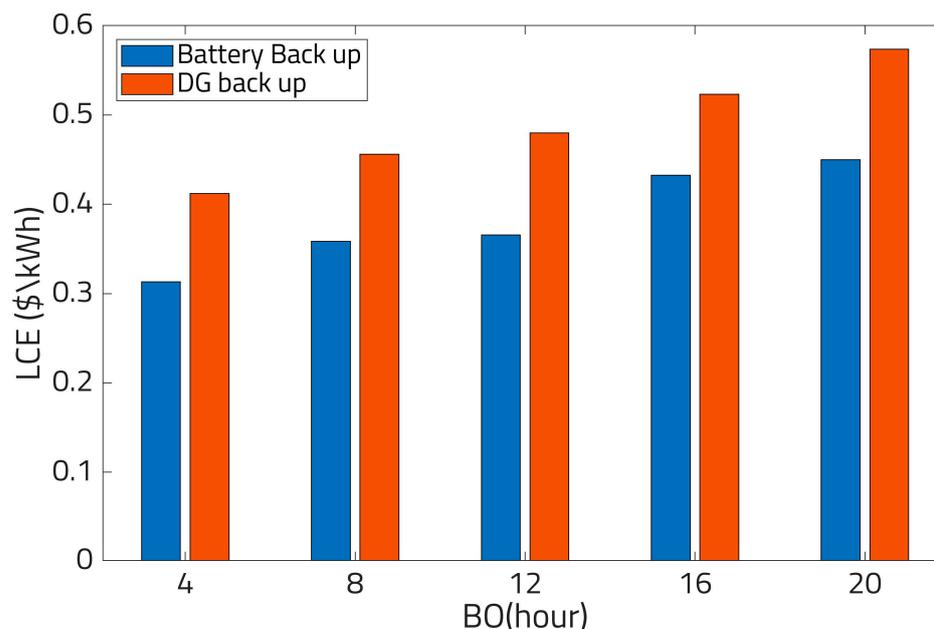
**Figure 15.** Comparison of levelized cost of energy of the battery backup system and the DG backup system. The chosen battery system is with priority dispatch,  $N_{bat} = 30$ , and  $C_{chrg} = 0.5 C$ . The DG system is sized based on the maximum load in the hospital, around 30 kW.
