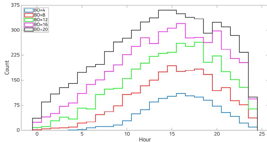
**Figure 17.** Histograms of the blackout distributions against the time of the day for different blackout durations for one year. The highest likelihood of blackout coincides with 4 pm and lowest is at midnight. Normal distribution is followed with standard deviation values between 4 and 9.
