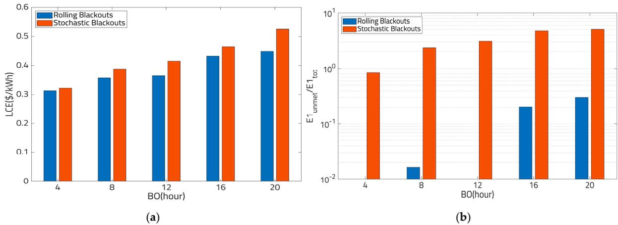
**Figure 18.** Comparison of the same system but with different blackout patterns: rolling (regular) blackouts (in blue) or stochastic blackouts with normal probability distribution function. (a) LCE and (b) normalized unmet critical load. The studied system has priority management,  $N_{bat} = 30$ , and  $C_{chrg} = 0.5 C$ . Note the logarithmic scale on subfigure (b).
