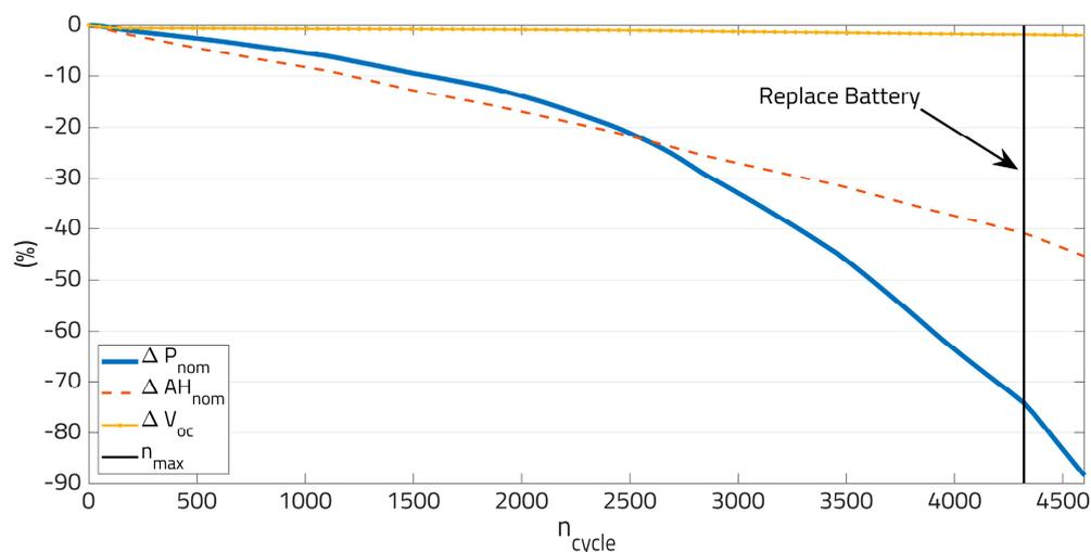
Figure 2. Aging characteristics for the Valence U1–12XP battery used in the model. Nominal capacity = 45 Ah at 12 V nominal with 576 Wh energy. The values are temperature-independent and correspond to room temperature conditions.
