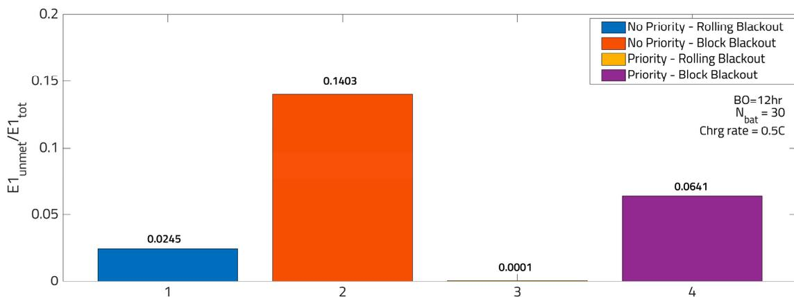
**Figure 19.** Comparison between priority and non-priority algorithms in the case of rolling blackout vs. block blackouts.
