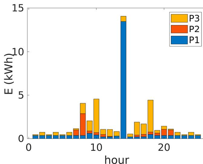
**Figure 4.** Hourly energy consumption of the studied hospital on a typical day showing the magnitude of the different priority loading. The large jump in the early afternoon coincides with using the X-ray machines, which have a capacity of 12 kW.
