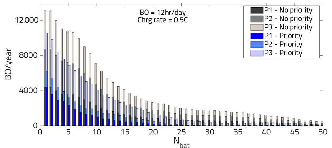
**Figure 9.** Comparison of blackout instances per year of priority and no-priority loading conditions as a function of the number of batteries in the system. In the no-priority scenario, every time a blackout occurs, all three loads are disconnected. With priority loading, P1 is prioritized.
