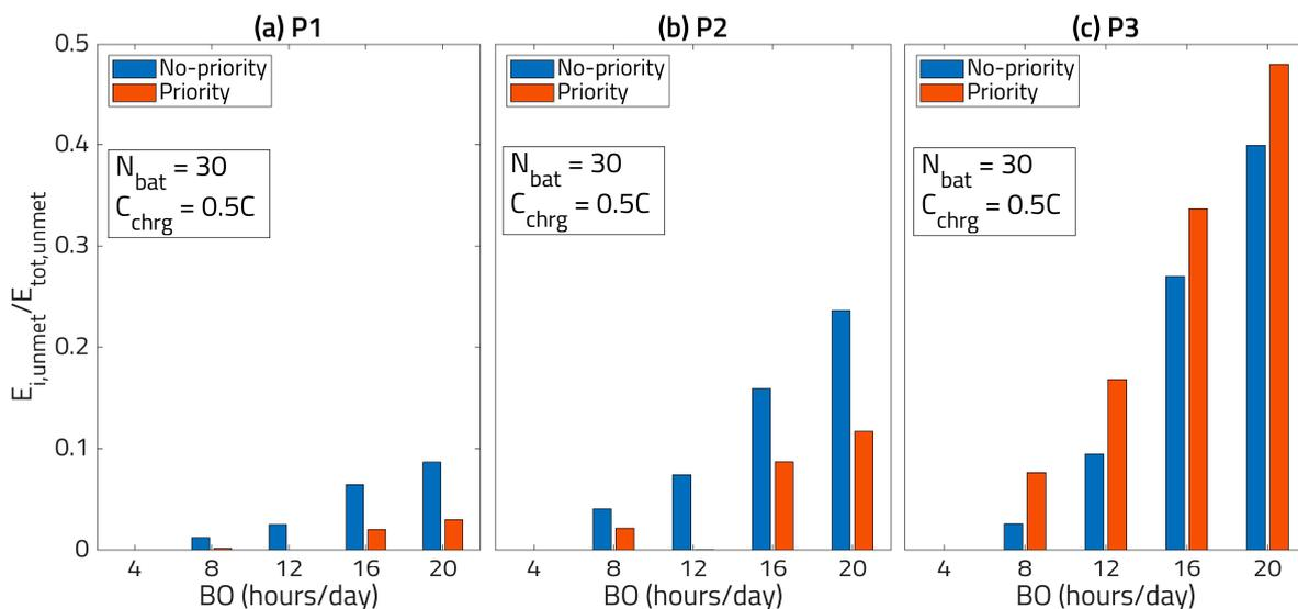
**Figure 12.** Energy ratio of different loads as a percentage of the total unmet load. The design point is taken at  $N_{bat} = 30$  and  $C_{chrg} = 0.5C$ . The priority dispatch strategy will reduce the ratio of P1 and P2 unmet loads at the expense of P3 unmet loads.
