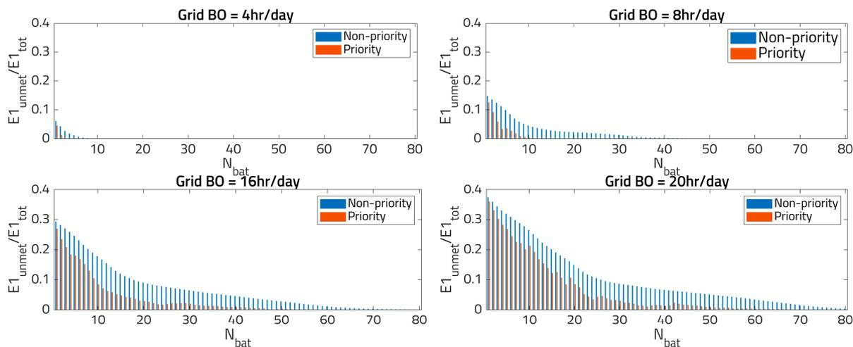
**Figure 13.** Ratio of unmet load P1 as a percentage of the total P1 load. All results are at  $C_{\text{chrg}} = 0.5 C$ . The priority dispatch strategy will reduce the ratio of P1 loads at the expense of P3 unmet loads.
