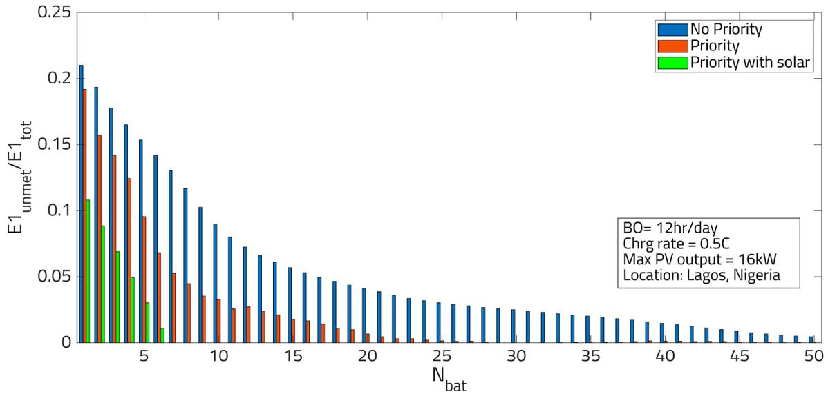
**Figure 16.** Normalized unmet energy for P1 load (E1) as a function of the system configuration and number of batteries in the system. This Figure is based on Figure 7 with the addition of the solar system to the priority load dispatch.
