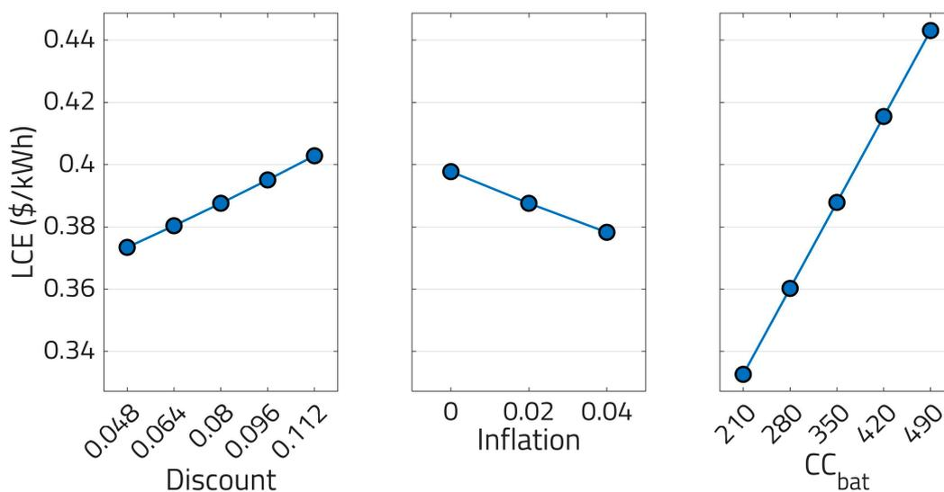
**Figure 20.** Main effects plot for the economic parameters effect on the levelized cost of energy of the battery backup system. Priority load management,  $N_{bat} = 30$ ,  $C_{chrg} = 0.5 C$ , and blackouts between 4–20 h are used to obtain the results.
