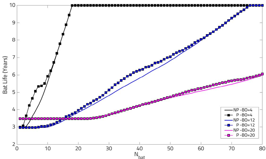
**Figure 14.** Effect of dispatch strategy on battery life at different blackout rates. NP = No-priority dispatch, P = Priority dispatch. Nominal battery life is assumed to be 10 years, regardless of cycling.
