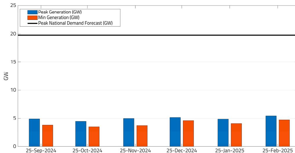
**Figure 5.** Peak and average national generation in Nigeria for selected days. The maximum daily load forecast is shown in the solid line at the top of the graph. The data are collected from the Nigerian Electricity System Operator [18].
