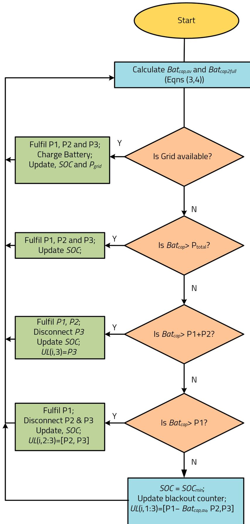
Figure 3. Energy dispatch strategy for three-tier load priority system with battery storage system.
