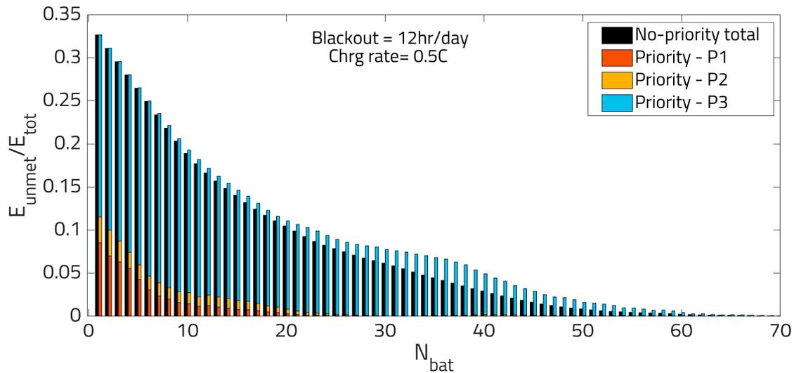
**Figure 8.** Ratio of unmet to total load as a function of the number of batteries in no-priority and priority loading.
