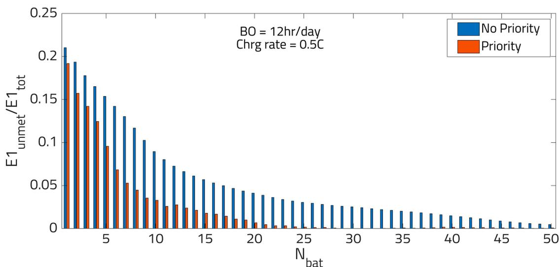
**Figure 7.** Normalized unmet energy for P1 load ( $E1$ ) as a function of the dispatch strategy and number of batteries in the system. In the non-priority case, the P1 unmet ratio is assumed to be the same as the ratio of the total unmet load to the total load in each timestep.
