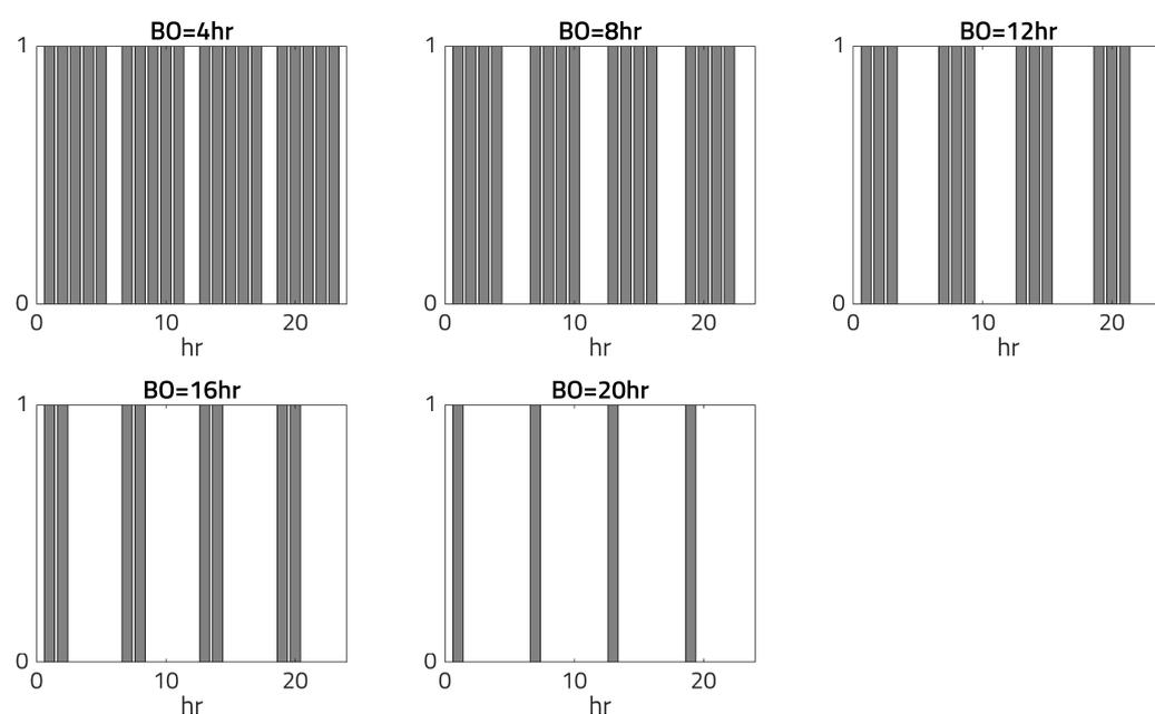
**Figure 6.** Typical blackout patterns with varying number of hours per day. A value of 1 means a grid is available, while a value of 0 means a blackout. Each day has four periods of blackouts.
