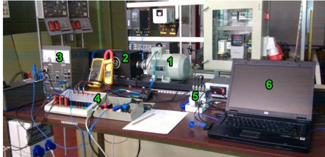
Fig. 5. Test bench: (1) Induction motor under test; (2) Magnetic powder brake; (3) Control unit; (4) Bespoke board with Hall effect transducers for current and voltage measurements; (5) DAQ board by National Instruments; (6) Laptop.
