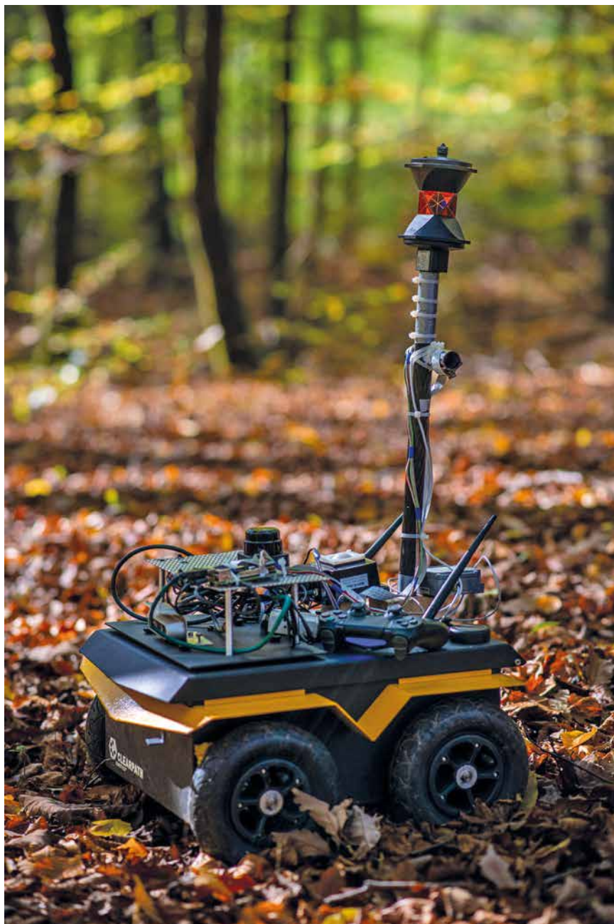
Figure 3. A common autonomous sensor box platform. This robot is designed to collect a range of different data including vegetation characteristics, tree locations and invertebrate data. Reproduced from Noskov et al. (2023) under Creative Commons licence CC BY 4.0.
