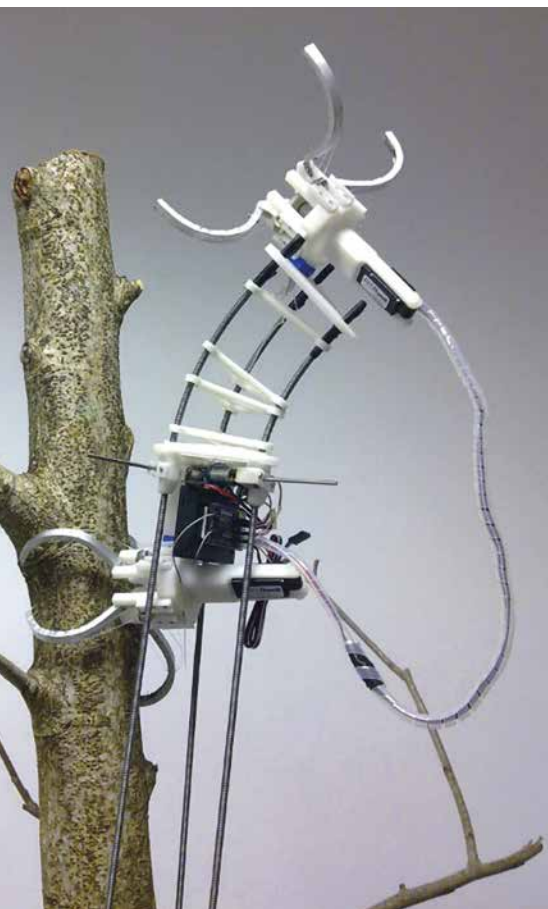
Figure 2. Treebot, a tree-climbing robot. This robot is highly specialised to climb trees but would struggle to adapt to other surfaces. Reproduced from Lam and Xu (2011) under Creative Commons licence CC BY 4.0.
