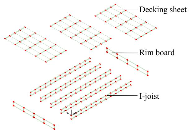
(a) Geometry of the individual structural elements
