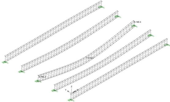
**Figure 6.1:** I-joists of Floor JJI 2 A under unit point load at the floor centre [3]
