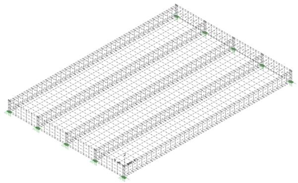
**Figure 3.2:** Mesh refinement of model (without spring stiffness at supports and joint elements) [3]
