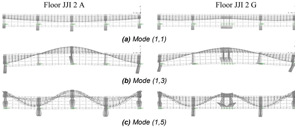
**Figure 5.2:** Mode shapes in transverse direction for the first three odd mode numbers of Floors JJI 2 A and G obtained from FEA [3]
