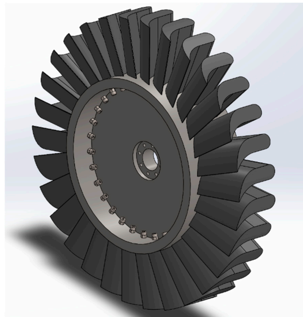
Figure 37. Selected bolted v2 turbine concept design.
