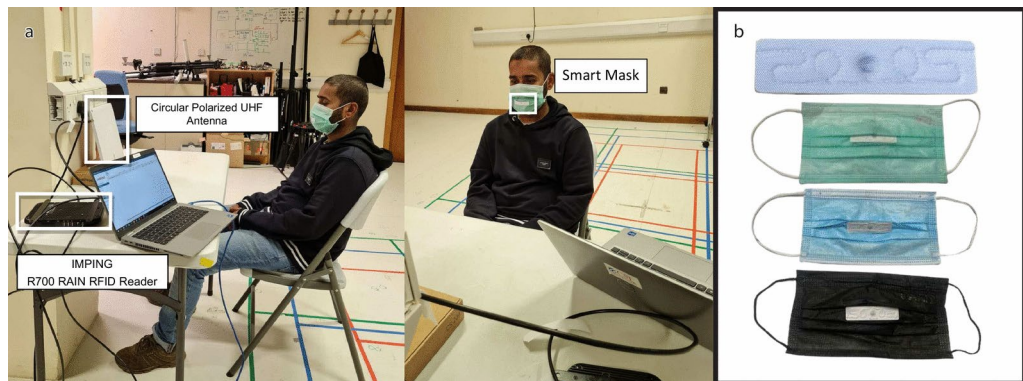
Fig. 4. Experimental setup of Lip-reading data collection using RFID-based smart mask. (a) Real experimental setup. (b) Color-thickness variants of smart masks used in the experimental setup.
