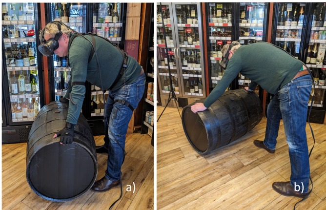
Fig. 5. (a) 90 th percentile operator while carrying out the bung removal OP assuming the posture PEI 2 ; (b) 90 th percentile operator while carrying out the racking warehousing OP assuming the posture PEI 3 .
