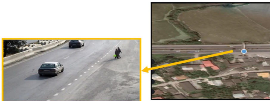
Fig. 1 – A snapshot of pedestrians crossing the road captured by a fixed video camera installed on the overpass (blue point) at the first location.
