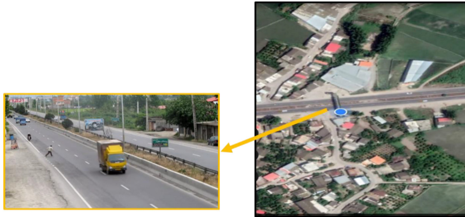
Fig. 2 – A snapshot of pedestrians crossing the path by a fixed video camera installed on the overpass (blue point) in the second location.
