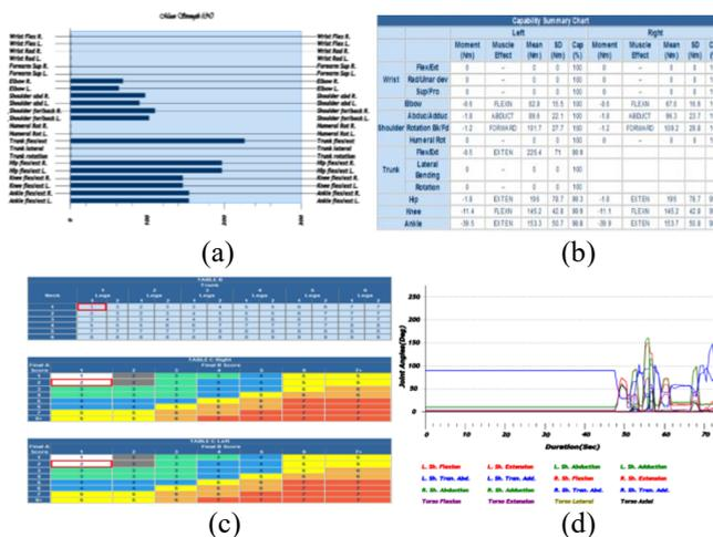
**Fig. 4.** (a) Static strength prediction (b) capability summary chart (c) RULA assessment chart (d) generic joint angle v/s time chart for worker 4.
