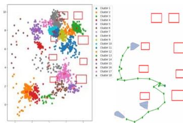
**Fig. 1.** (a) Clustering using Hierarchical Dendrogram (b) Worker Path and Dwell regions on the workplace.
