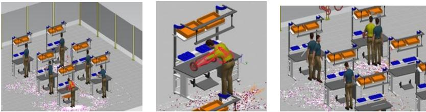
**Fig. 2.** A pictorial depiction showcasing the tasks performed by workers during the assembly process and visualising continuous ergonomic assessment and worker interactions in the digital twin
