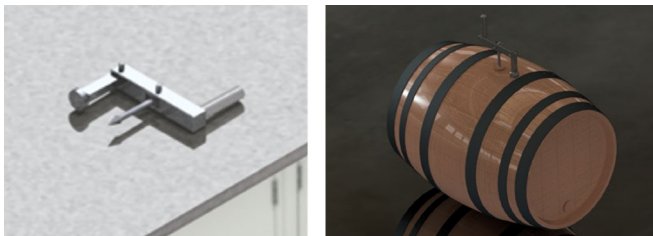
Fig. 2. Bung removal tool,[1].
