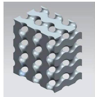
**(a) Typical Gyroid Structure (b) TPMS Architecture Scaffold**
