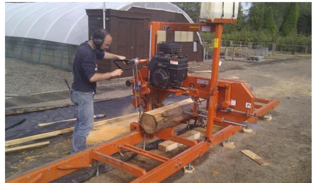
**Figure 2.** Processing of a western red cedar log with a portable sawmill.
