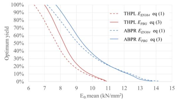
**Figure 7:** Graph based on modulus of elasticity for THPL and ABPR samples showing the difference in yields by using equation (1) or (3).  $E_{0,mean}$  is the mean of the population achieving the correspondent value.
