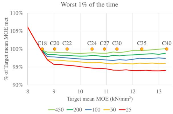
**Figure 10:** Simulation of the uncertainty for the mean MOE of different sample size.
