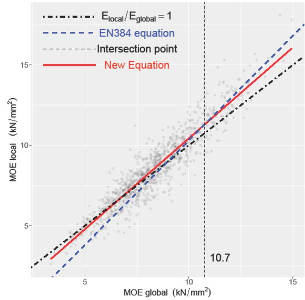
**Figure 6.** Relationship between  $E_{local}$  and  $E_{global}$  as proposed by EN384 and as derived locally in this study. The vertical dashed line denotes the intersection point of the lines described by these relationships. The directly proportional relationship is also shown.
