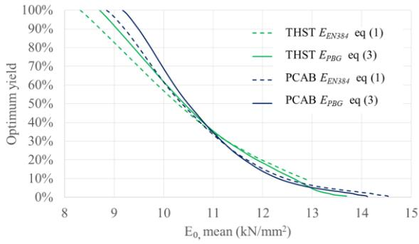
**Figure 8:** Graph based on modulus of elasticity for THST and PCAB samples showing the difference in yields by using equation (1) or (3).  $E_{0,mean}$  is the mean of the population achieving the correspondent value.
