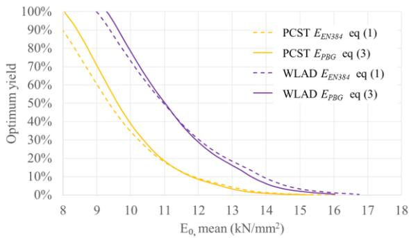
**Figure 9:** Graph based on modulus of elasticity for PCST and WLAD sample showing the difference in yields by using equation (1) or (3).  $E_{0,mean}$  is the mean of the population achieving the correspondent value.
