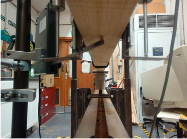
**Figure 3.** Transducers for measurement of  $E_{global}$  (bottom face) and  $E_{local}$  (side faces).
